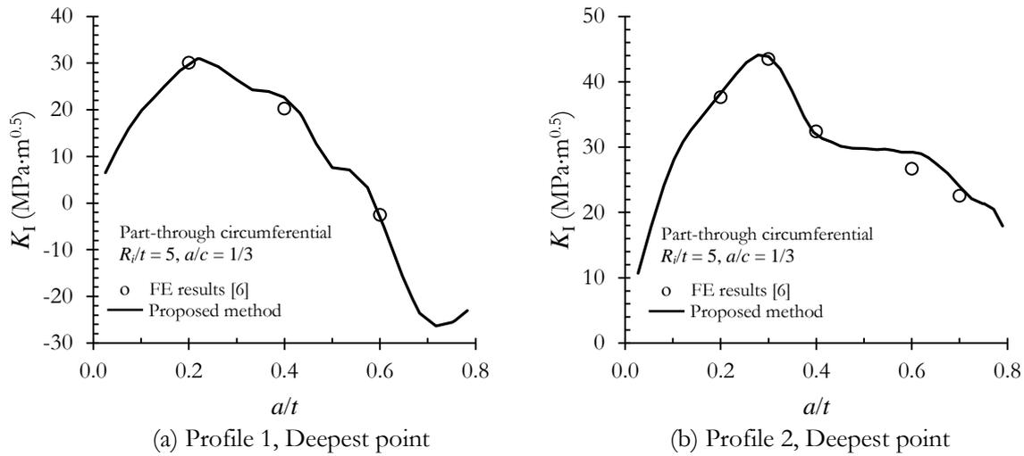
Fig. 9. Comparison of  $K_I$  estimated by piecewise linear approximation with FE solutions for case no. 2.
