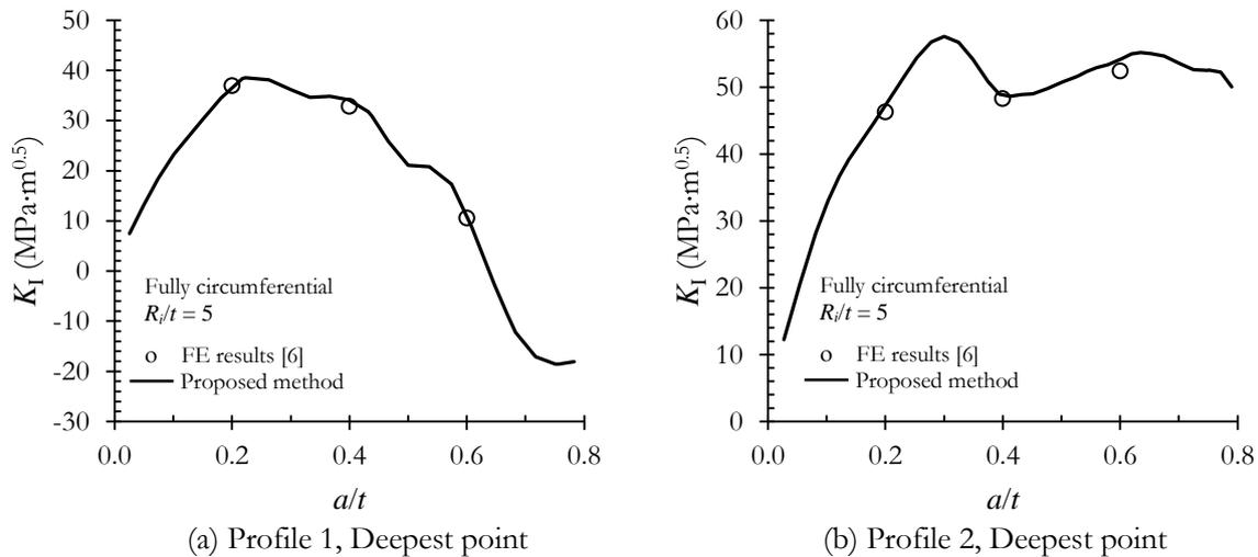
Fig. 11. Comparison of  $K_I$  estimated by piecewise linear approximation with FE solutions for case no. 4.
