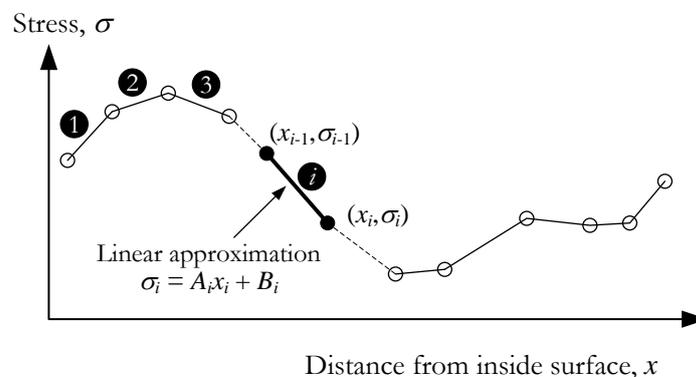
Fig. 6. Approximation of stress between two discrete points by a straight line.
