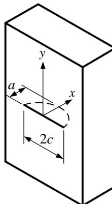
Fig. 2. Plate with semi-elliptical surface crack.
