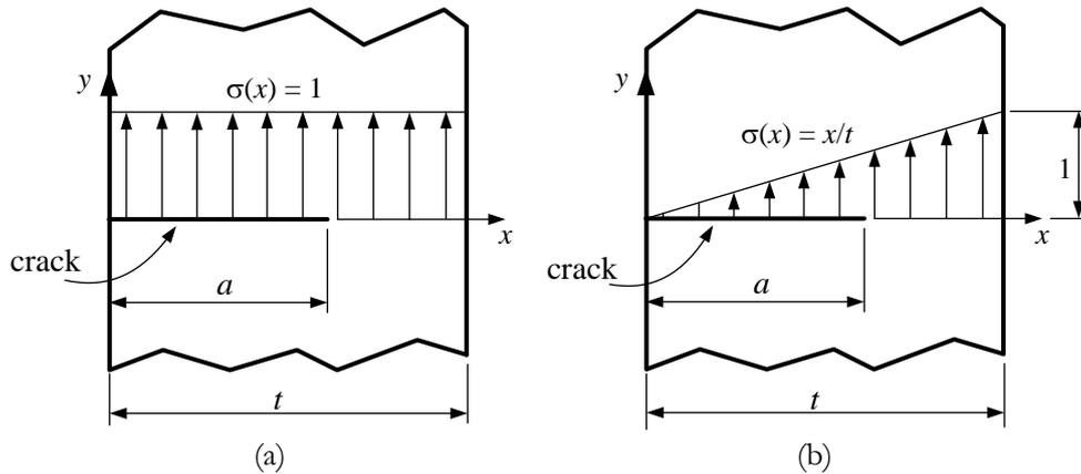
Fig. 3. Two references loading cases used for determining weight function coefficients: (a) Uniform stress distribution, (b) Linear stress distribution.
