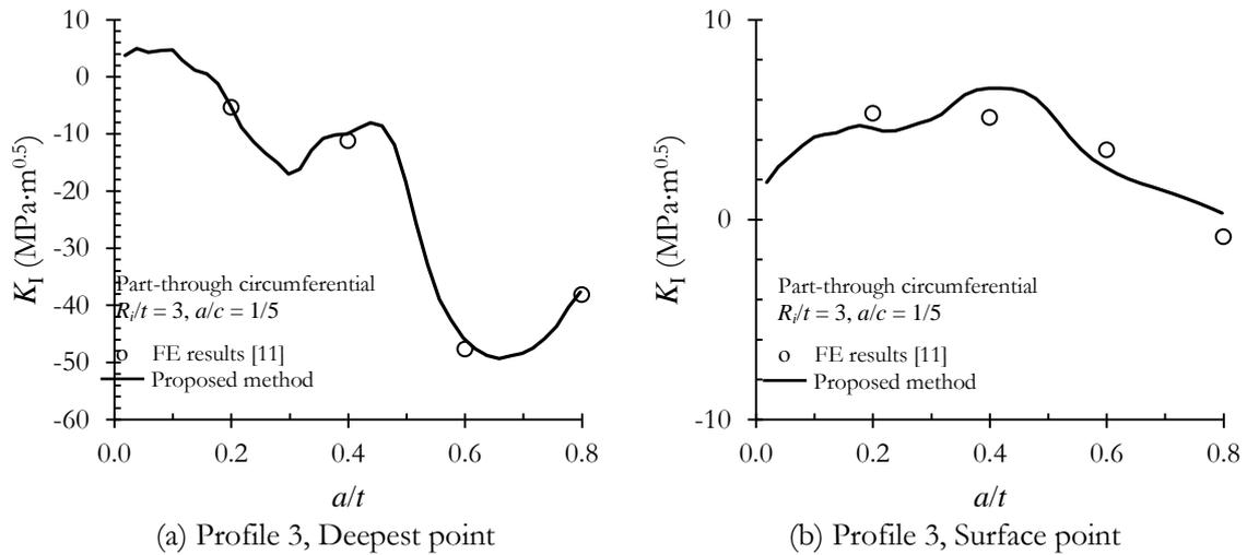
Fig. 10. Comparison of  $K_I$  estimated by piecewise linear approximation with FE solutions for case no. 3.
