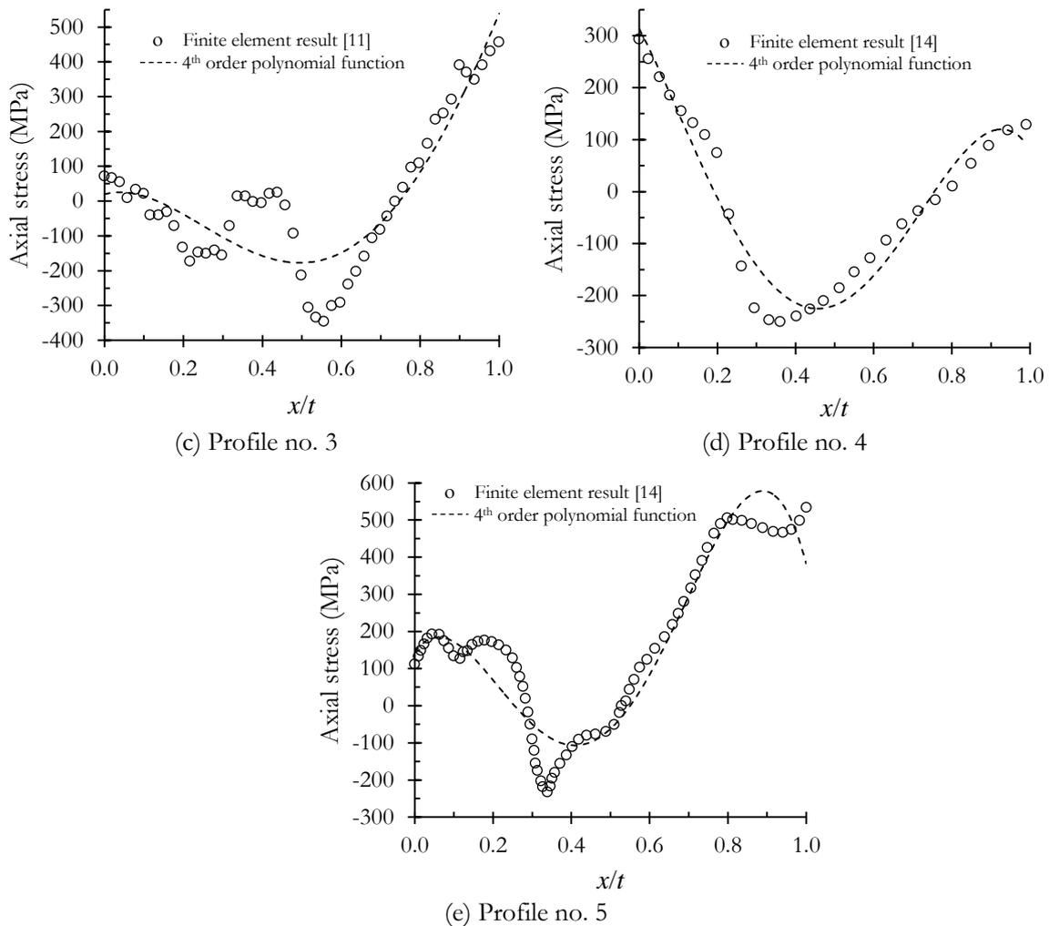
Fig. 7. Weld residual stress profiles used in validation of a proposed weight function and a piecewise linear approximation of stress profile.
