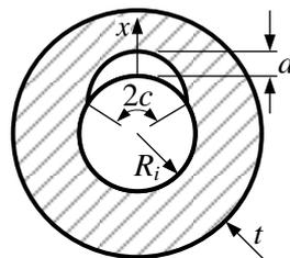
Fig. 4. A cylinder with internal part-through circumferential crack.
