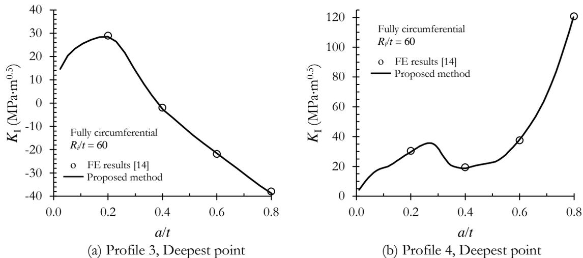
Fig. 12. Comparison of  $K_I$  estimated by piecewise linear approximation with FE solutions for case no. 5.
