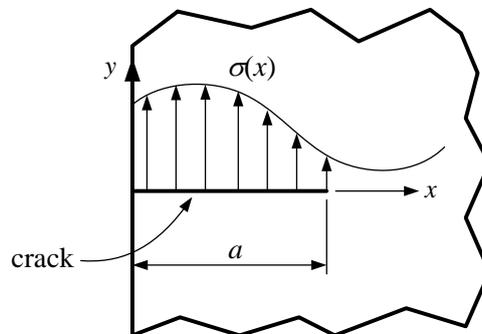
Fig. 1. Two-dimensional body with edge crack subjected to arbitrary stress distribution on the crack plane.
