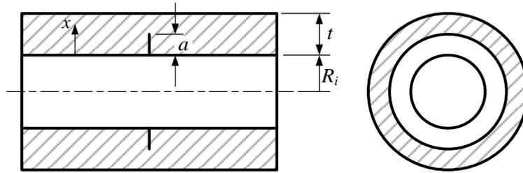
Fig. 5. A cylinder with internal fully circumferential crack.
