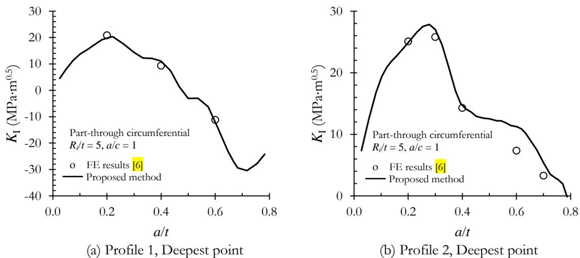
Fig. 8. Comparison of  $K_I$  estimated by piecewise linear approximation with FE solutions for case no. 1.
