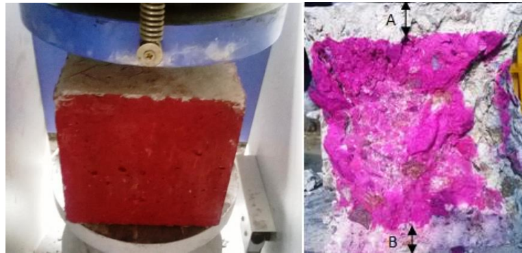
Fig. 3. (a) Compressive strength of concrete; (b) Measure of depth of carbonation.
