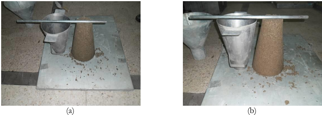
Fig. 8. (a) Slump test of CD 100% and (b) Slump test of 8:12:20:60 (% by weight) mixture.
