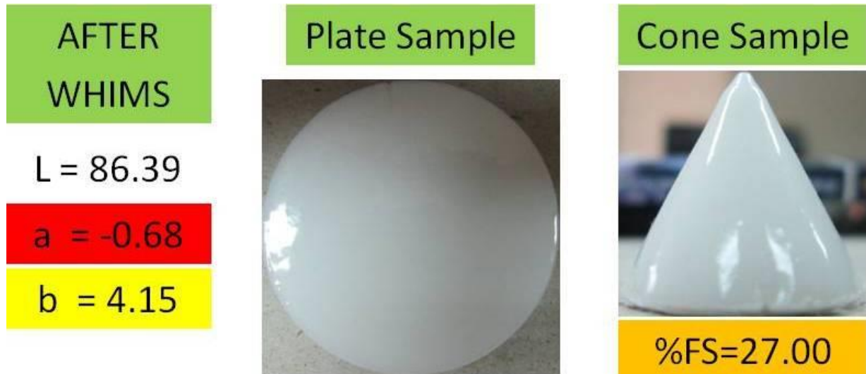
Fig. 11. Fire test result of the after WHIMS feldspar.
