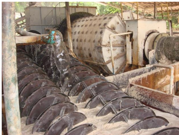
Fig. 4. Arrangement of the feldspar grinding circuit.
