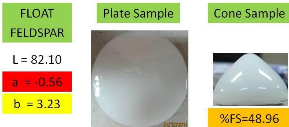
Fig. 12. Fire test result of the final product feldspar.
