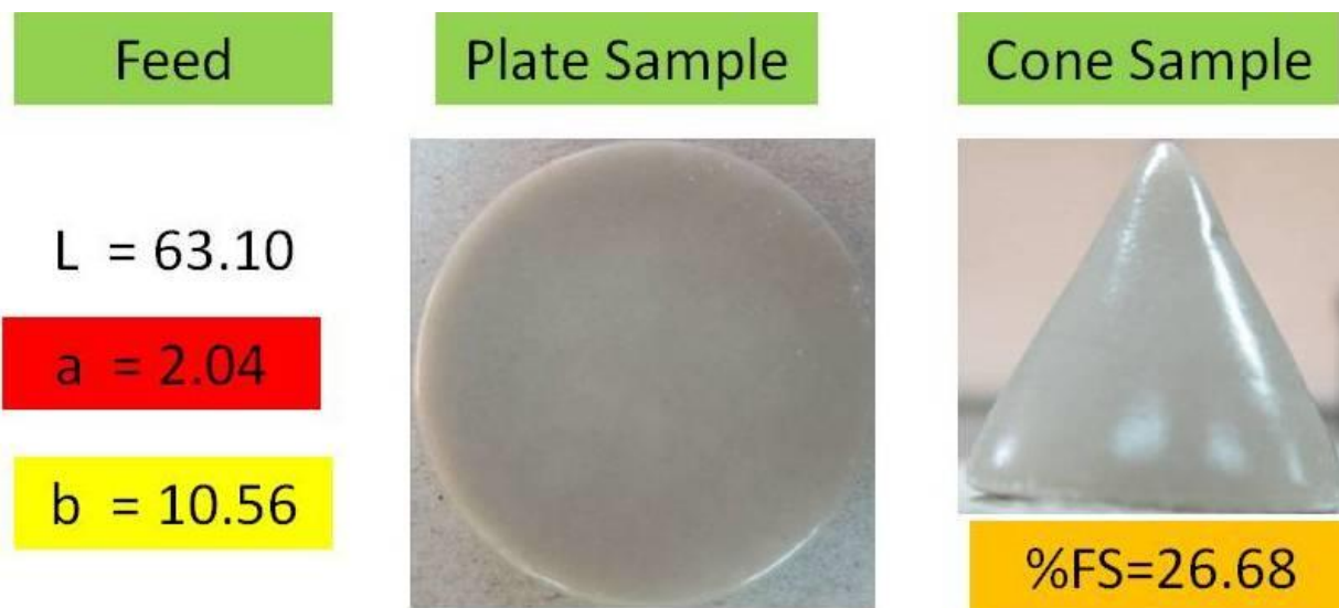
Fig. 10. Fire test result of the feed ore feldspar.
