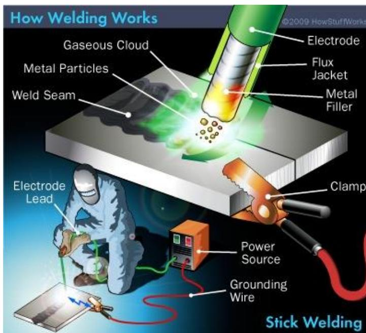
Fig. 2. The process of arc welding (HowStuffWorks [8]).
