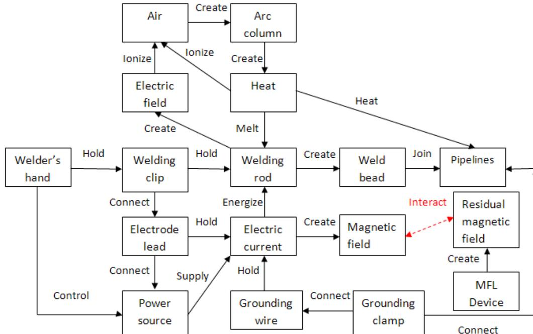
Fig. 4. Function Model of the pipeline welding system.
