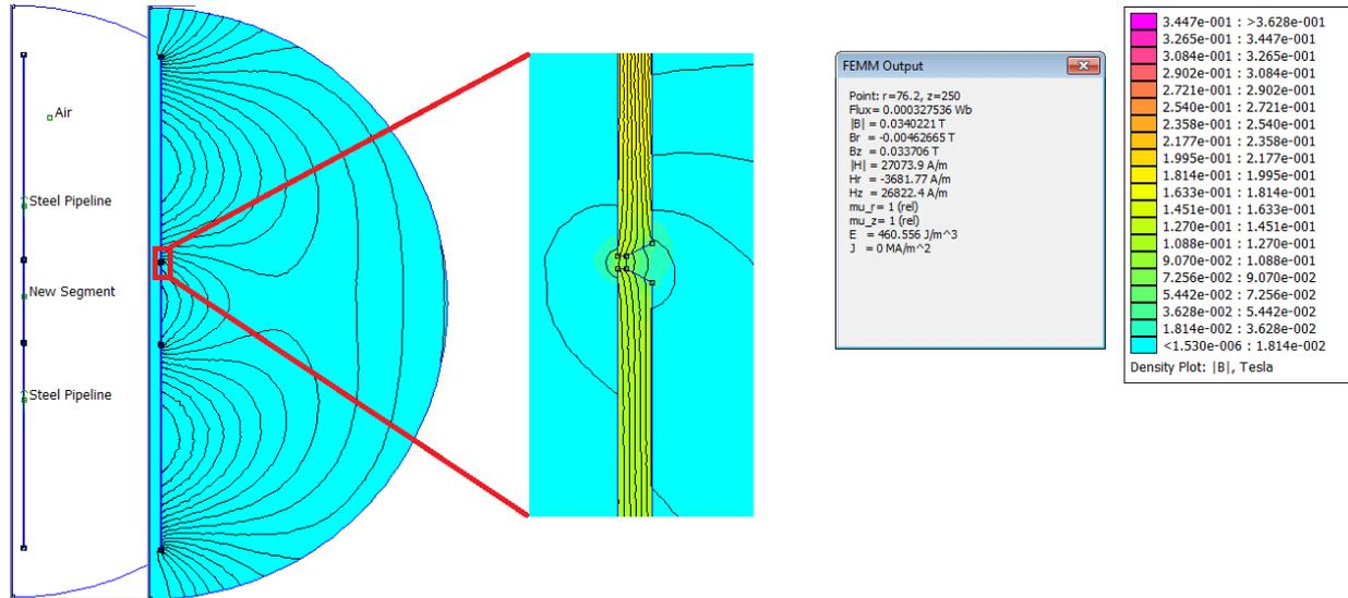
Fig. 21. Magnetic field simulation with no compensation.
