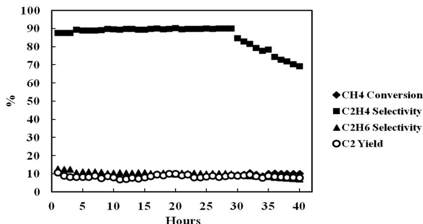
Fig. 13. Stability test of P-Na<sub>2</sub>WO<sub>4</sub>-Mn/YSZ catalyst in SOFC reactor at 1123 K.
