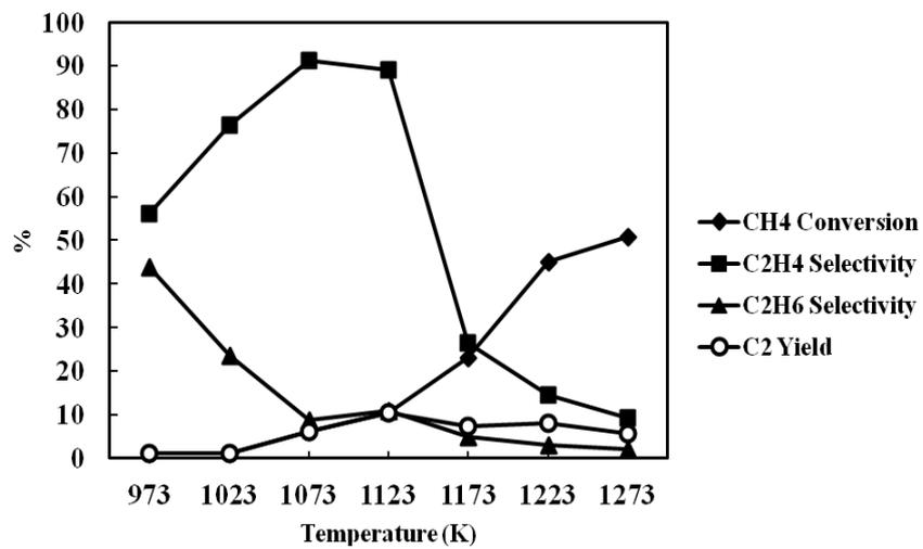
Fig 12. Performance of P-Na<sub>2</sub>WO<sub>4</sub>-Mn/YSZ catalyst in SOFC reactor.
