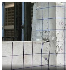
(d) The shear, flexure, diagonal compression of the column-flanking wall joints
