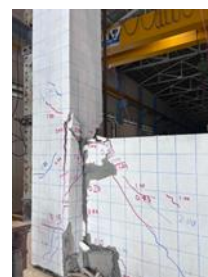
(Left) (Right) (c) Diagonal compression cracks of column-flanking wall joints
