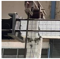
(c) The flexural and shear cracks of column-beam joint
