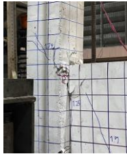
(d) The shear, flexure, diagonal compression of the column-flanking wall joints
