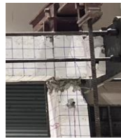
(c) The flexural and shear cracks of column-beam joint
