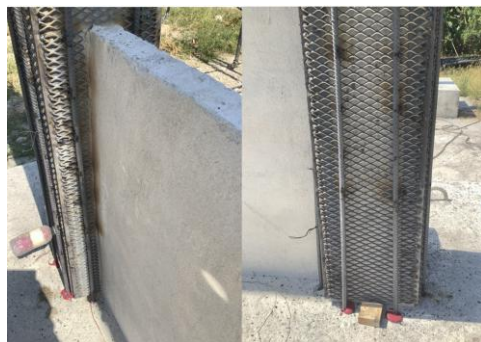
(c) Detail of external bars embedded into the concrete base
