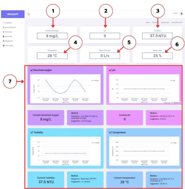
Fig. 13. Real-time water quality data from various sensors in aquaculture ponds.
