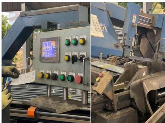
Fig. 11. A rebar cutting and bending machines equipped with QR codes and barcode readers
