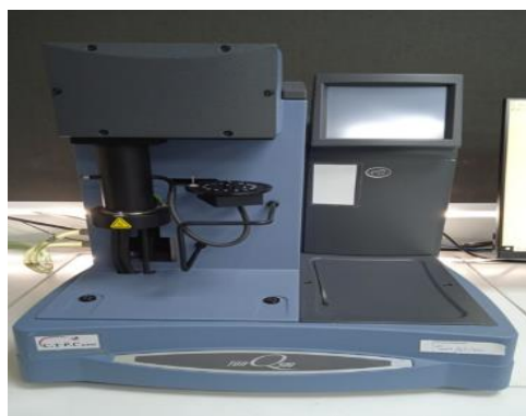
Fig. 5. Q500 Thermogravimetric analyser from TA Instrument.
