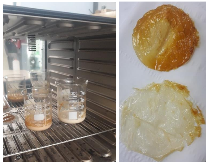
Fig. 2. Collected films through thermal extraction via the use of a laboratory oven.
