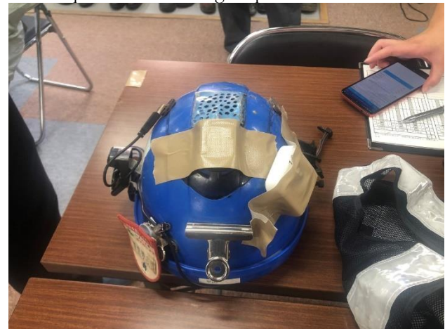
Fig. 2. Installation of sensors on helmets and connection status via Bluetooth.
