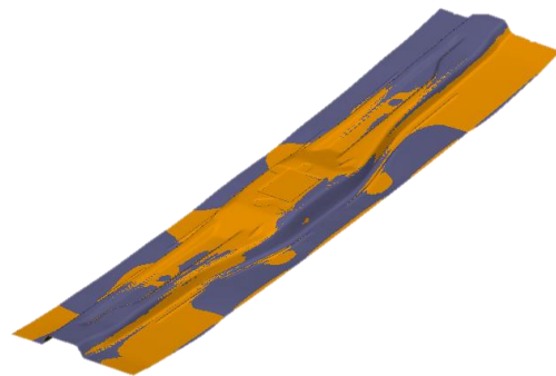
Fig. 5. Scanned model and simulation result at same position with Bestfit.
