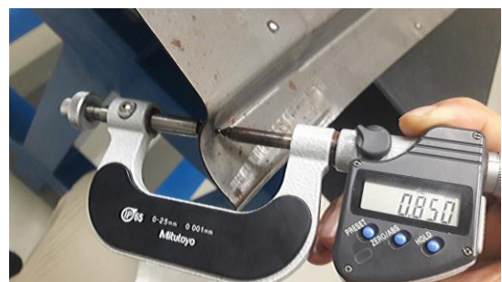
Fig. 22. The thickness measuring tool is measuring at sample point 1.
