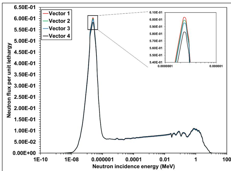
Fig. 4. Neutron flux per unit lethargy of PCMSR with various fuel vectors.
