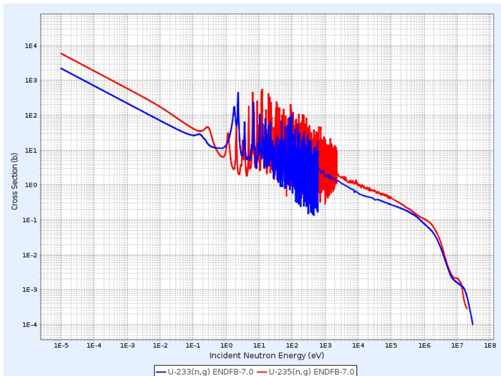
Fig. 3. Neutron capture cross section of U-233 (blue) and U-235 (red). The cross section was taken from Evaluated Nuclear Data Library (ENDF)/B-VII.0.
