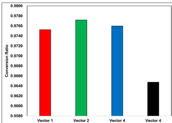
Fig. 7. Conversion ratio of PCMSR with various fissile vector.
