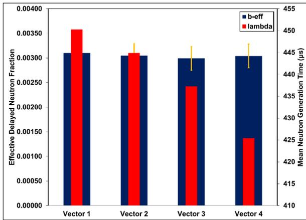
Fig. 5. Kinetic parameters of PCMSR with various fuel vectors.
