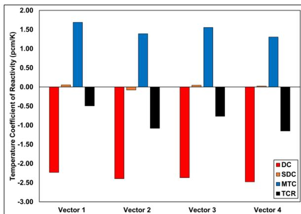
Fig. 6. Temperature coefficient of reactivity for PCMSR with different U-233 purity.
