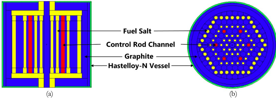
Fig. 2. PCMSR Reactor Core Model (a) Axial view; (b) Radial view.
