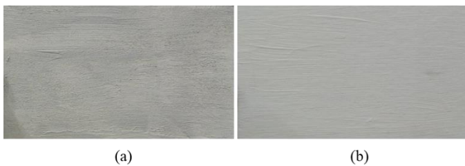
Fig. 6. The color of the paint finishes after drying 24 hours: (a) gray for sample Ca-1 (with Ca(OH)_2 ) and (b) white for sample Ca-2 (without Ca(OH)_2 ).
