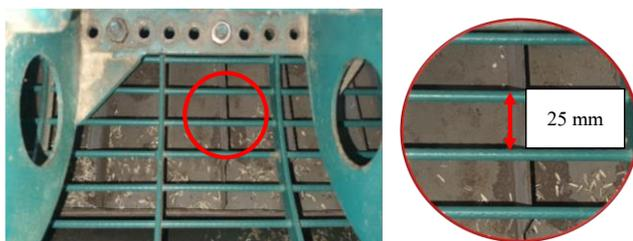
Fig. 5. Concave rod clearance.
