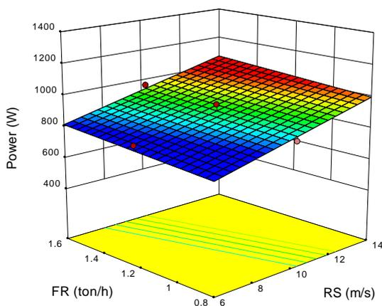
Fig. 10. Graphical response surface affecting power.
