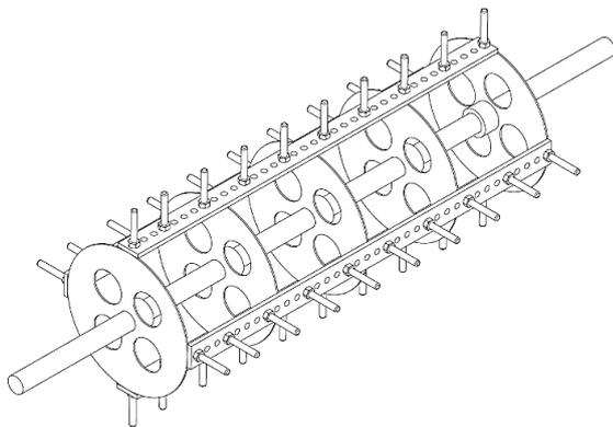
Fig. 3. Structural design of spiked teeth.
