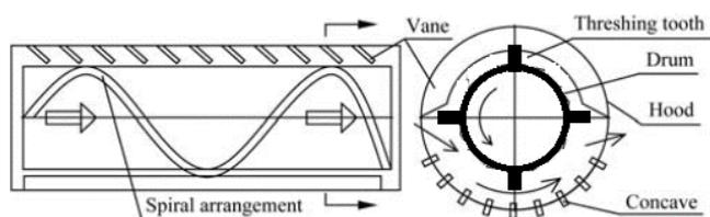
Fig. 1. Axial flow threshing characteristics.
