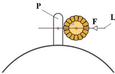
Fig. 2. The acting force between the spike-tooth and the sunflower.
