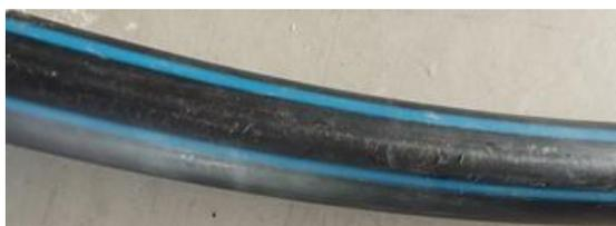
Fig. 2. Pipe of PEHD (PE100).
