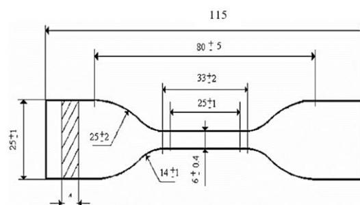
Fig. 4. Shape of the HDPE-PE100 pipe specimens.
