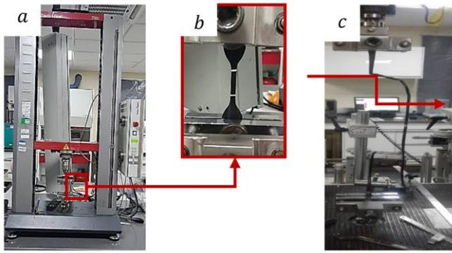
Fig. 5. Tensile test of the specimens of HDPE-PE100 pipes—a) Test start; b) Extension; c) fracture.
