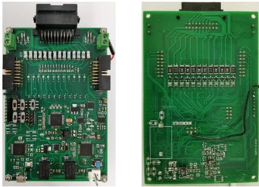
Fig. 14. Actual board of the proposed flexible BMS (left) top layer (right) bottom layer.
