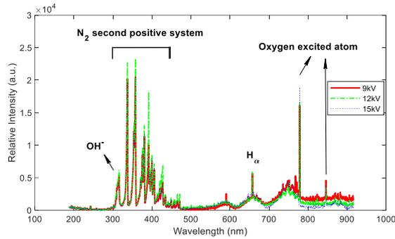
Fig. 5. OES of air plasma during the soil treatment.
