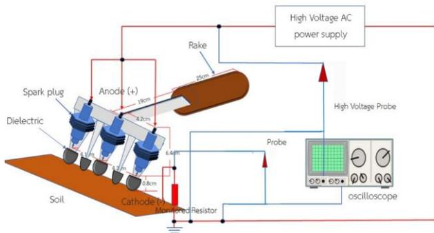
Fig. 1. The schematic drawing of experimental setup for a spark plug plasma.
