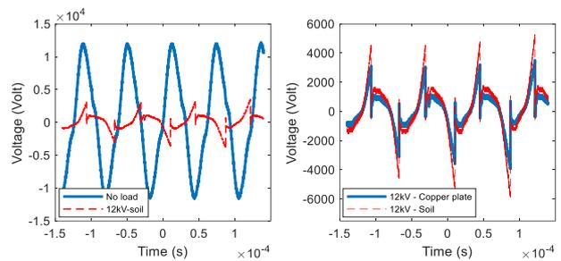
Fig. 3. Comparison of voltage waveform characteristics at 12 kV supplied voltage with the gap distance of 4 mm between a) no-load and soil load (electrode), and b) copper plate and soil electrode.
