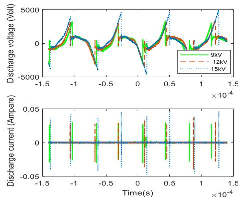
Fig. 4. Discharge voltage and current characteristics during soil treatment at different supplied voltages.
