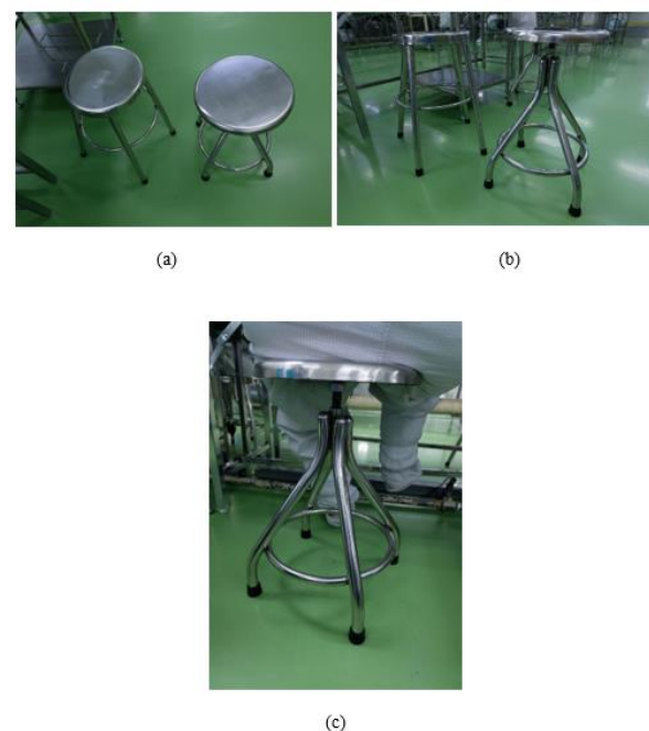
Fig. 9. The comparison of a new design of the work chair and the original chair: (a) top view, (b) side view and (c) in service.
