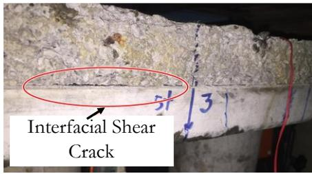
a) Interfacial shear failure
