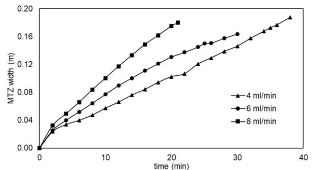
Fig. 4. Mass transfer zone width in a fixed bed column at flow rate of 4, 6, and 8 ml/min.
