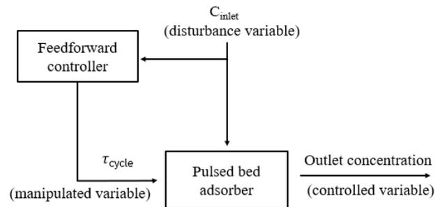
Fig. 1. Block diagram of feedforward control of pulsed bed adsorption column.
