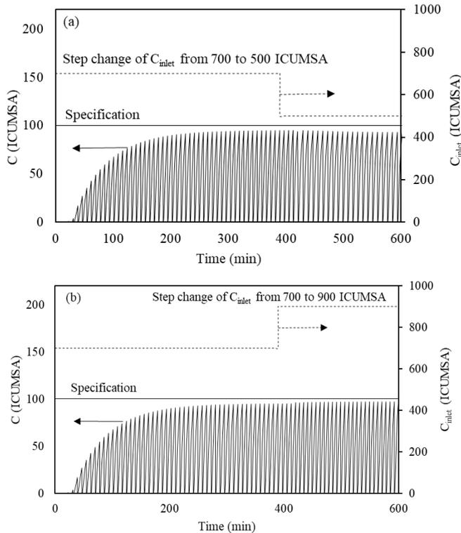
Fig. 10. The predicted performance of pulsed bed model for step change at flow rate 6 ml/min (a) cycle time adjusted with the delay of 5 cycles for a step change of inlet concentration from 700 to 500 ICUMSA and (b) cycle time adjusted with the delay of 5 cycles for a step change of inlet concentration from 700 to 900 ICUMSA.
