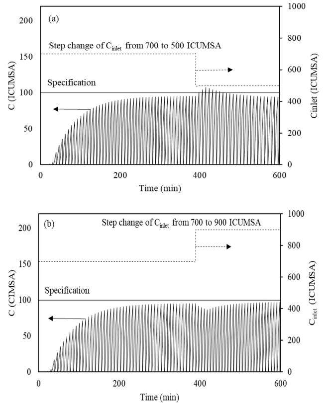
Fig. 9. The predicted performance of pulsed bed model for step change at flow rate 6 ml/min (a) cycle time adjusted immediately for step change of inlet concentration from 700 to 500 ICUMSA and (b) cycle time adjusted immediately for step change of inlet concentration from 700 to 900 ICUMSA.
