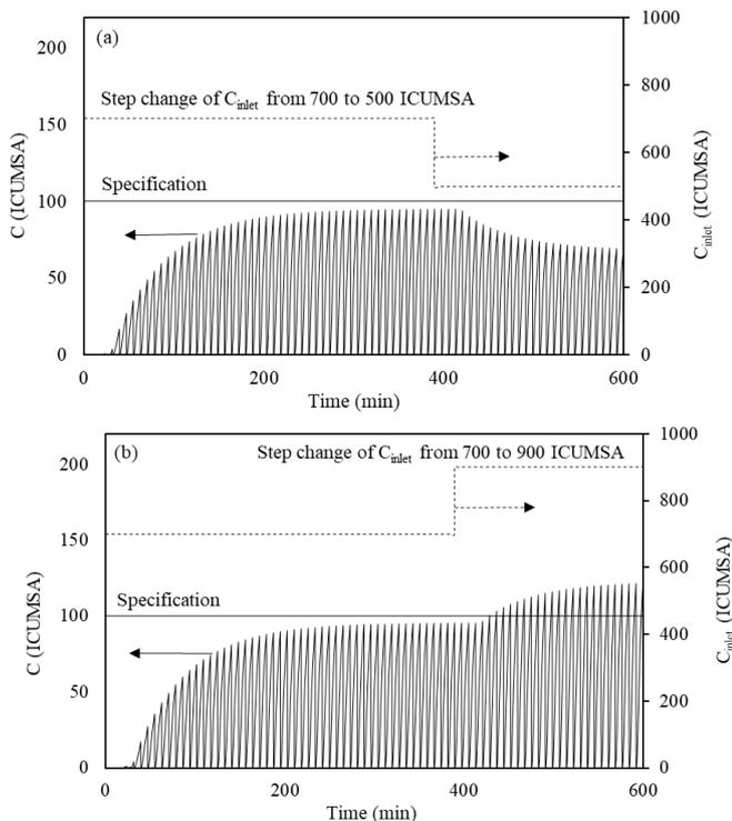
Fig. 8. The predicted performance of pulsed bed column at constant cycle time of flow rate 6 ml/min (a) inlet
