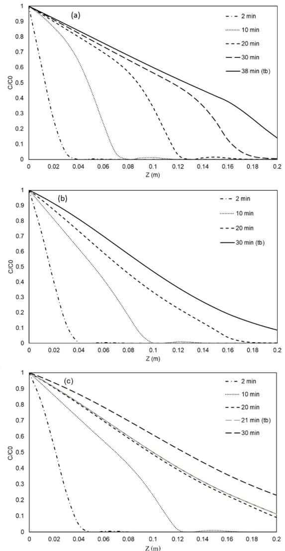
Fig. 3. Concentration profiles inside a fixed bed column obtained from a model at different flow rates (a) 4 ml/min (b) 6 ml/min and (c) 8 ml/min.
