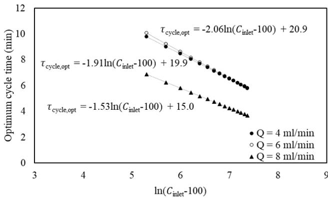
Fig. 7. Relationship between inlet concentration and optimum cycle time of pulsed bed adsorber column at feed flow rates of 4, 6 and 8 ml/min.
