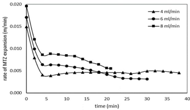
Fig. 5. Rate of mass transfer zone (MTZ) expansion in fixed bed at flow rate of 4, 6 and 8 ml/min.
