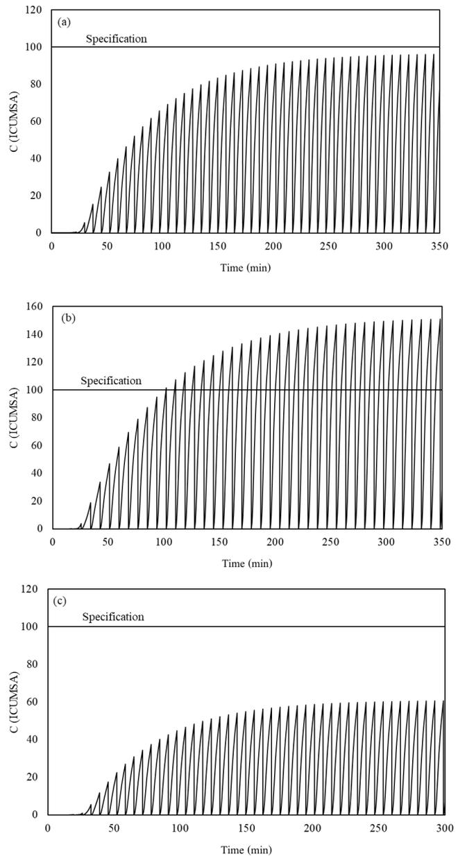
Fig. 6. The predicted performance of pulsed bed column at inlet concentration 700 ICUMSA of feed flow rate 6 ml/min. (a) optimum cycle time of 7.68 min (b) cycle time < optimum cycle time and (c) cycle time > optimum cycle time.
