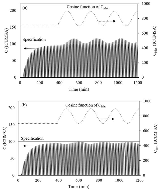
Fig. 11. The predicted performance of pulsed bed column of inlet concentration changes of 700 ICUMSA to cosine function (a) without feedforward control and (b) cycle time adjusted with the delay of 5 cycles.
