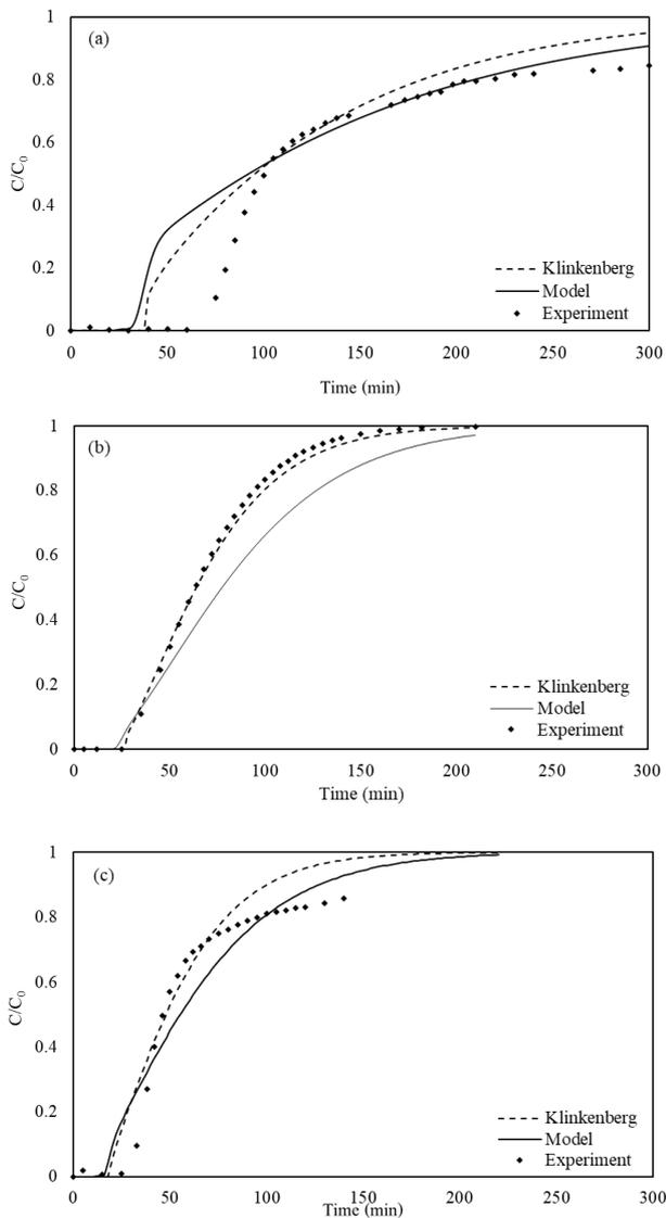
Fig. 2. Comparison between breakthrough curve from experiment, Klinkenberg and the model of fixed-bed column at different flow rates (a) 4 ml/min (b) 6 ml/min and (c) 8 ml/min.
