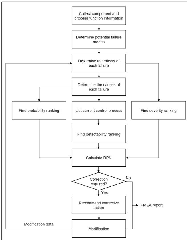
Fig. 11. Standard FMEA procedure (Adapted from Pillay and Wang [93]).
