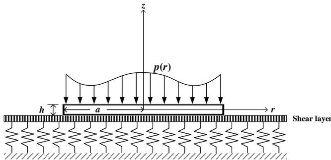
Fig. 1. Circular nanoplate on two-parameter elastic substrate medium.
