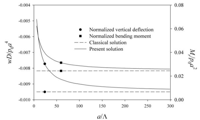
Fig. 9. Variations of normalized central deflection and normalized bending moment with the normalized plate radius  $a/\Lambda$  for a uniformly loaded circular nanoplate with simple support on two-parameter elastic substrate.
