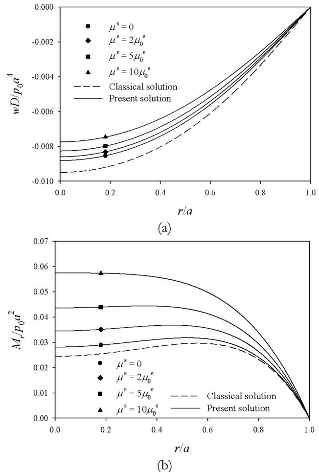
Fig. 7. Profiles of (a) normalized vertical deflection and (b) normalized bending moment of a uniformly loaded circular nanoplate with simple support on two-parameter elastic substrate for different values of  $\mu^s$ .
