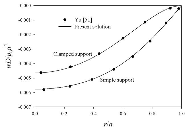
Fig. 2. Comparisons for normalized deflection of a circular plate on two-parameter elastic substrate medium without surface energy effects.
