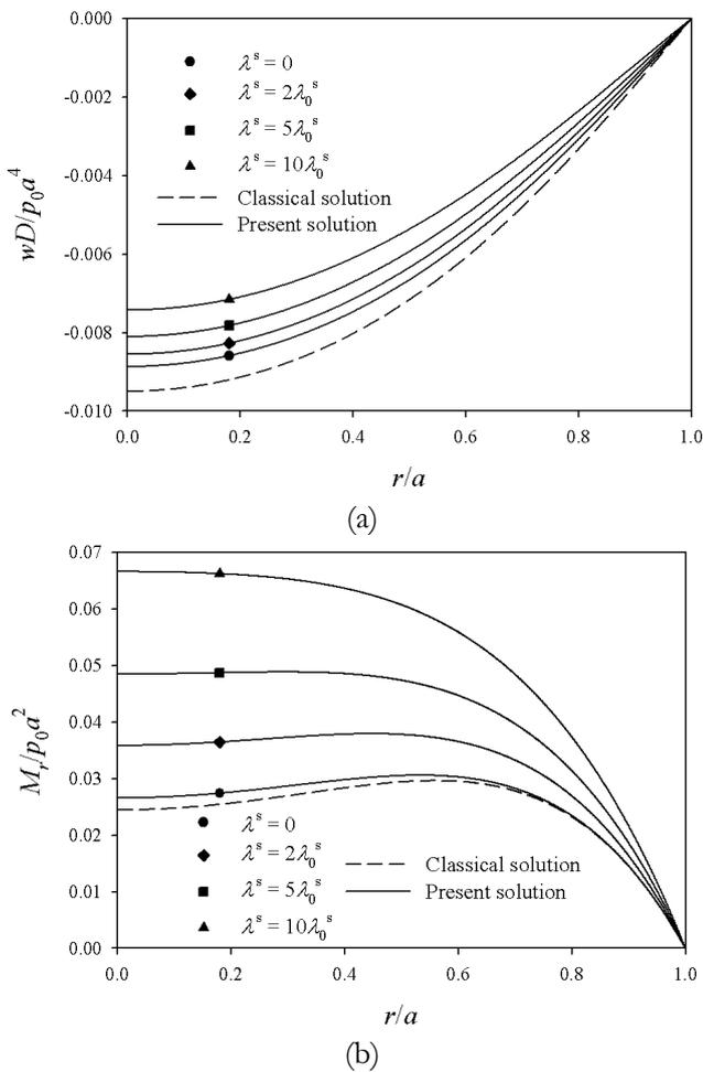
Fig. 6. Profiles of (a) normalized vertical deflection and (b) normalized bending moment of a uniformly loaded circular nanoplate with simple support on two-parameter elastic substrate for different values of  $\lambda^s$ .
