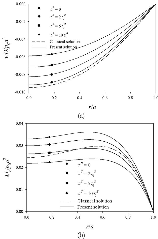
Fig. 8. Profiles of (a) normalized vertical deflection and (b) normalized bending moment of a uniformly loaded circular nanoplate with simple support on two-parameter elastic substrate for different values of  $\tau^s$ .
