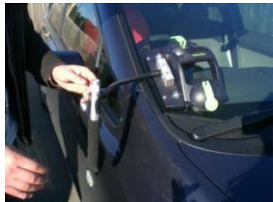
Fig. 4. Microphones are mounted at the arch of front right and left wheels.
