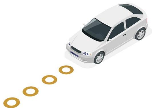
Fig. 9. Multiple Segmented Coils for Dynamic Charging.
