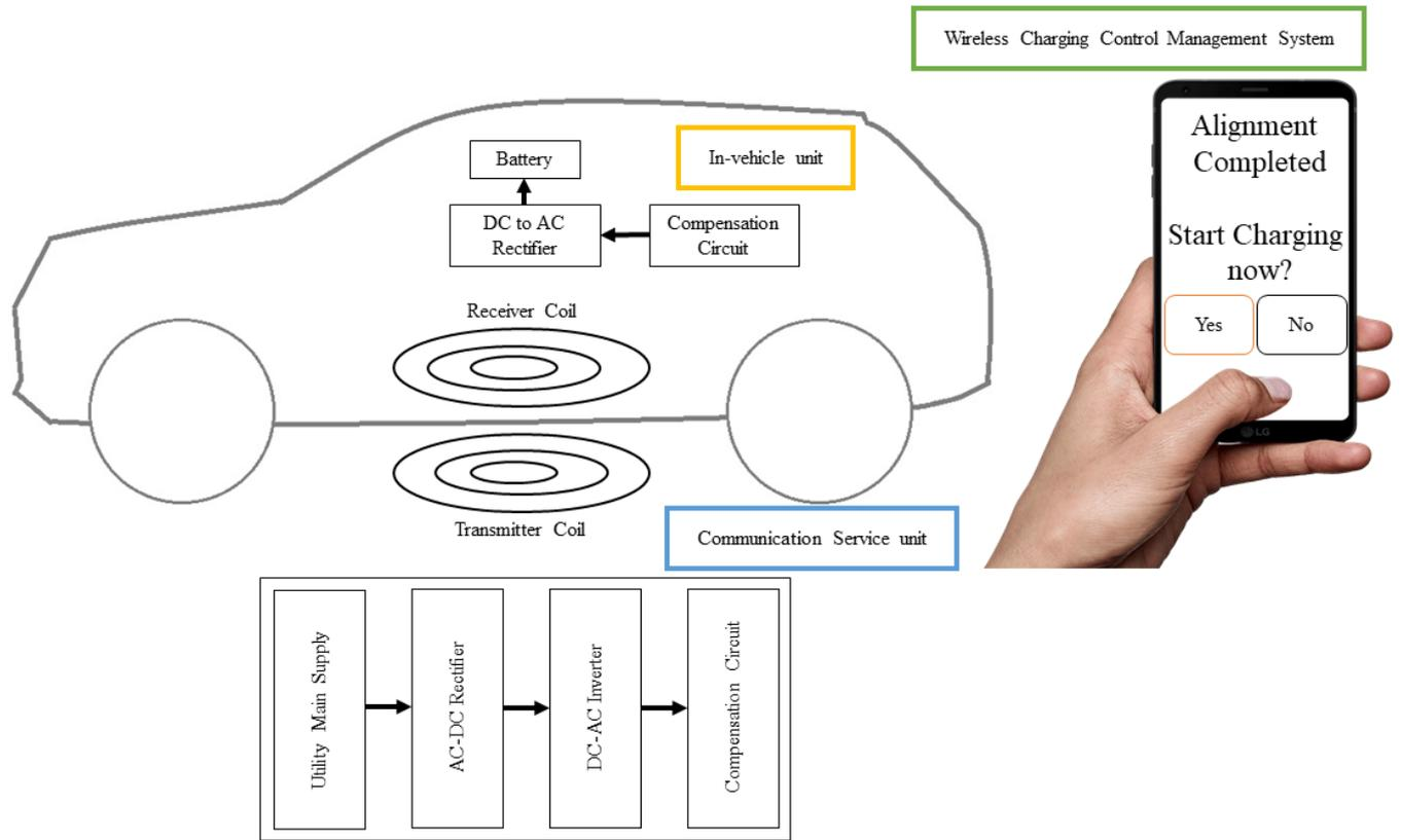
Fig. 1. Structure diagram of typical WPT system for EVs.
