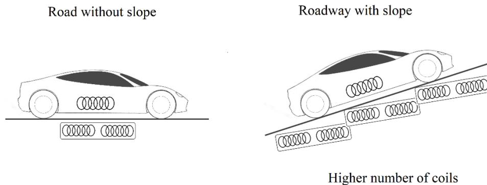
Fig. 3. Difference between Coils on a Roadway with and without a gradient.
