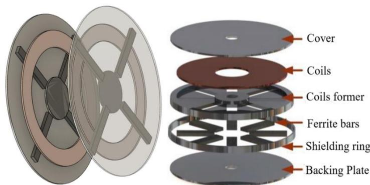
Fig. 4. A Circular Pad Structure.
