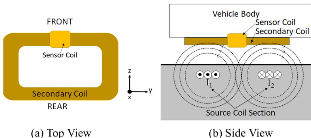
Fig. 11. Advanced autonomous coil alignment system using one sensor coil.
