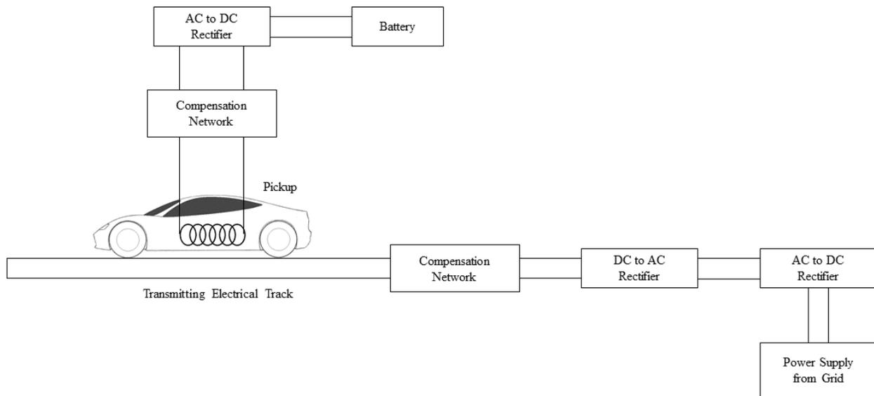
Fig. 8. Single-Coil Long Transmitter Track.
