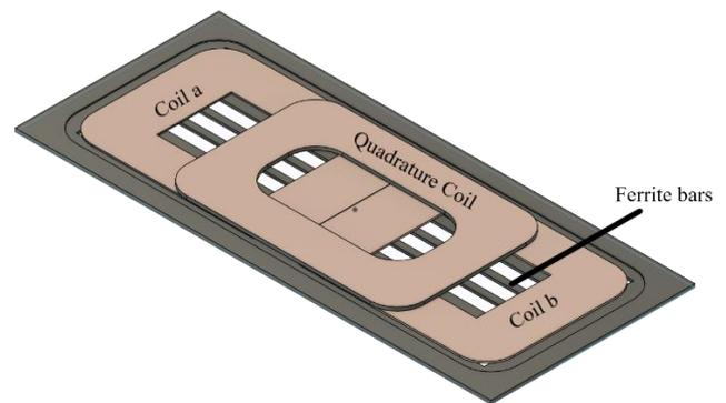
Fig. 6. Double-D Quadrature coil design.
