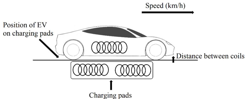
Fig. 2. Three factors of Wireless Charging of EV.
