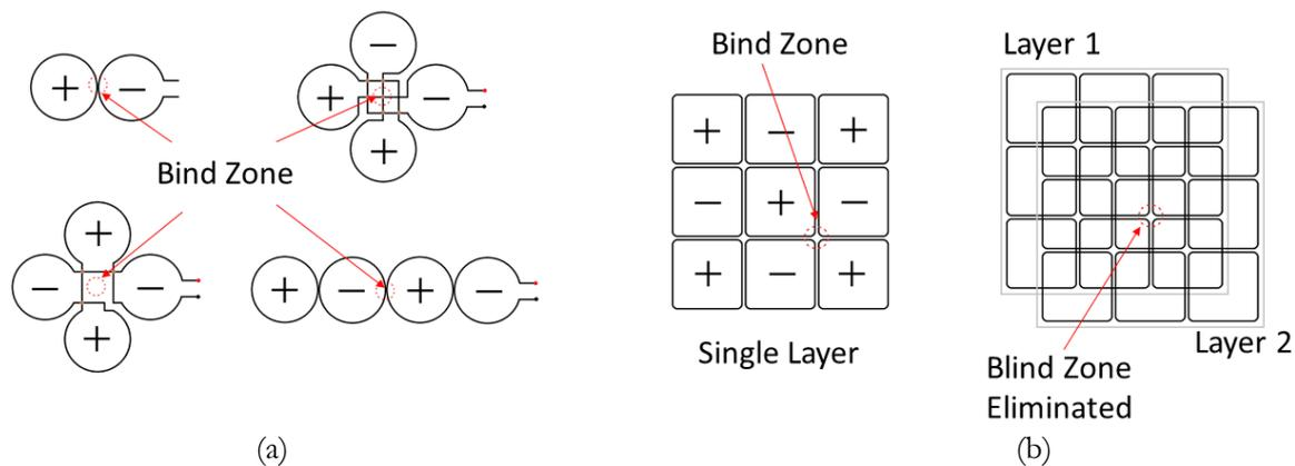
Fig. 10. (a) Single-layer, (b) Two-layer structure of Overlapped coils configuration.
