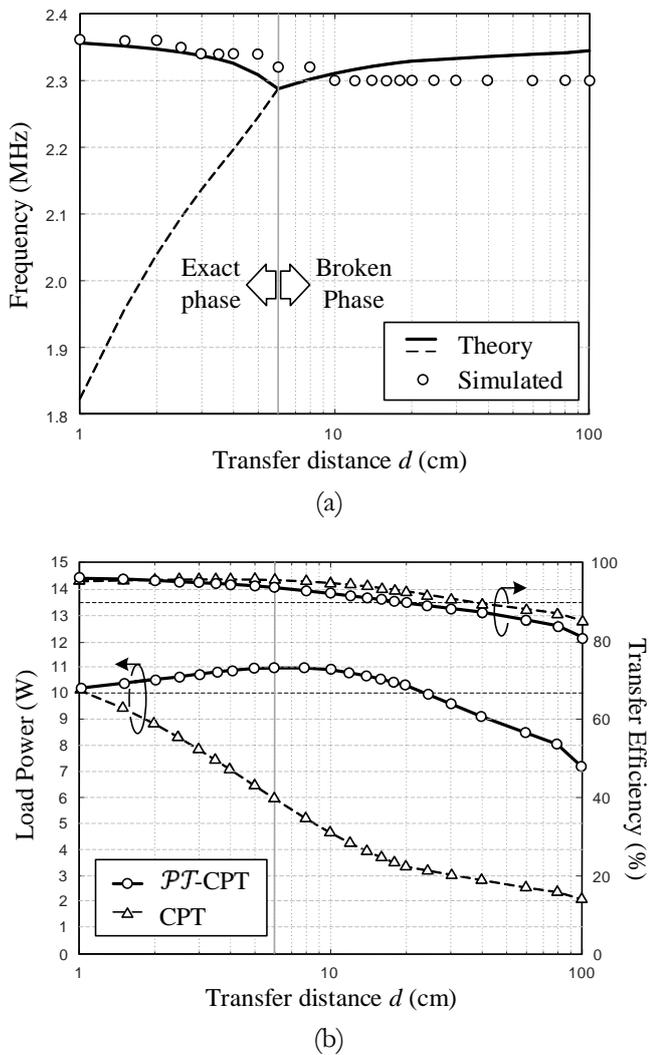
Fig. 4. Demonstrated nonlinear  $\mathcal{PT}$ -CPT system. (a) simulated and theoretical eigen-frequencies versus distance (b) simulated load power and efficiency versus distance in comparison with conventional CPT.
