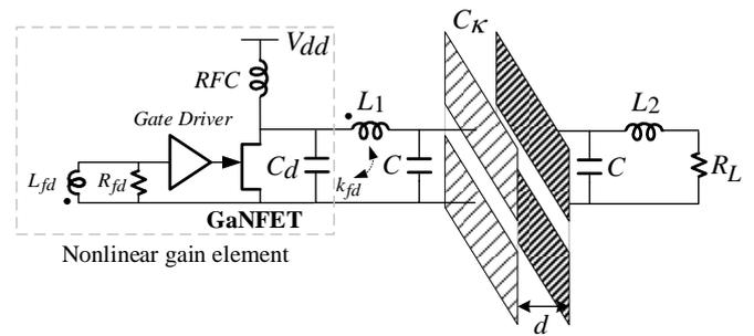
Fig. 3 Practical nonlinear  $\mathcal{PT}$ -CPT schematic using positive-feedback class-E switching power amplifier and four-plate coupling structure.
