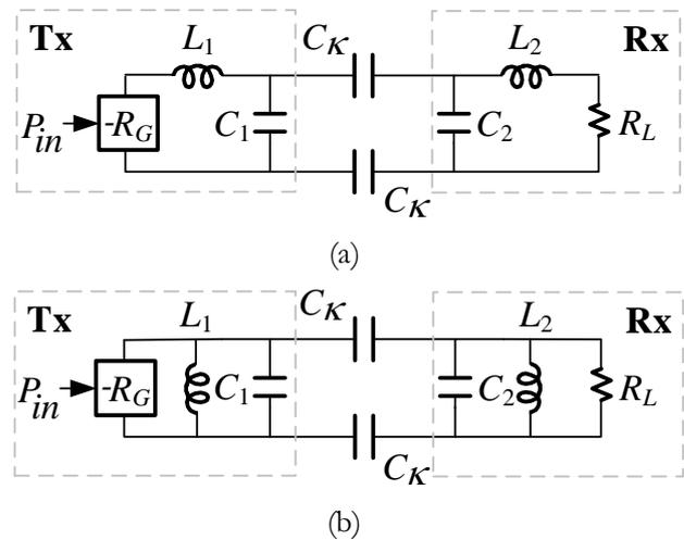
Fig. 1.  $\mathcal{PT}$ -symmetric capacitively coupled resonant system (a) coupled Tx-Rx series resonators, (b) coupled Tx-Rx parallel resonators.
