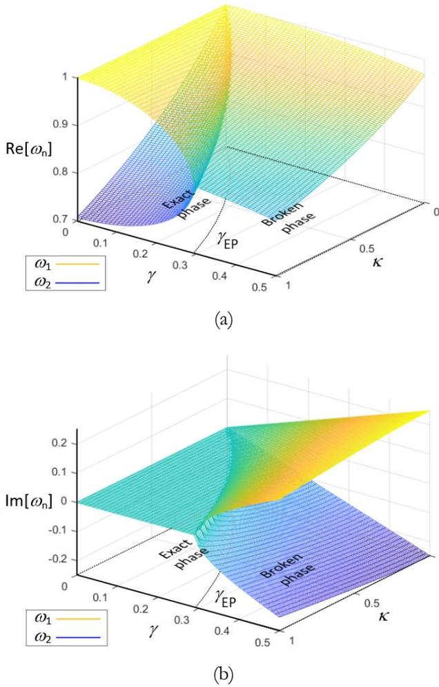
Fig. 2. Eigen-frequency characteristics versus non-Hermiticity parameter  $\gamma$  and coupling factor  $\kappa$  in  $\mathcal{PT}$ -CPT using series resonators. (a) real part, (b) imaginary part with exact and broken phase boundary.
