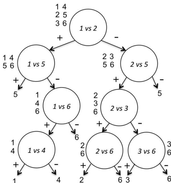
Fig. 1. The Illustration of the binary tree of SVM (BTS). Some data classes may be scattered at some node and appear in more than one leaf node. [13]
