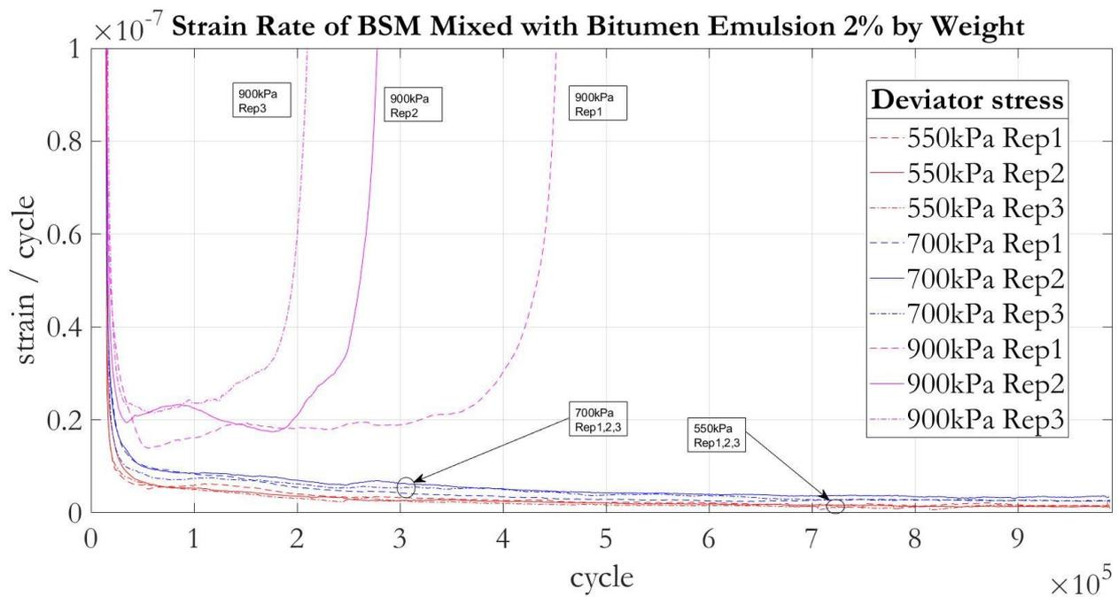
Fig. 10. Relationships between the number of repeated load cycles and the permanent strain rate of the 2% BSM specimens.
