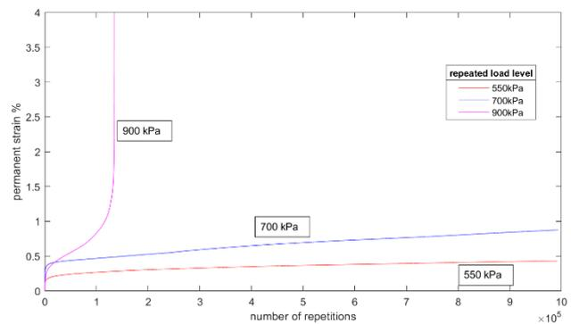
Fig. 3. An example of permanent axial strain responses under different levels of repeated loads.
