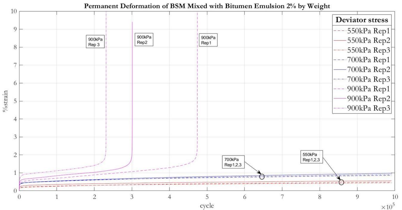
Fig. 9. Relationships between the number of repeated load cycles and the accumulated permanent strain of the 2% BSM specimens.
