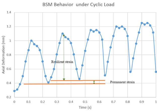
Fig. 6. Axial deformation of a BSM specimen recorded from a displacement transducer during the test.
