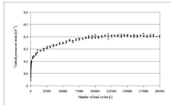
Fig. 2. Relationships between the number of repeated load cycles and permanent vertical strain under the plastic shakedown pattern [19].
