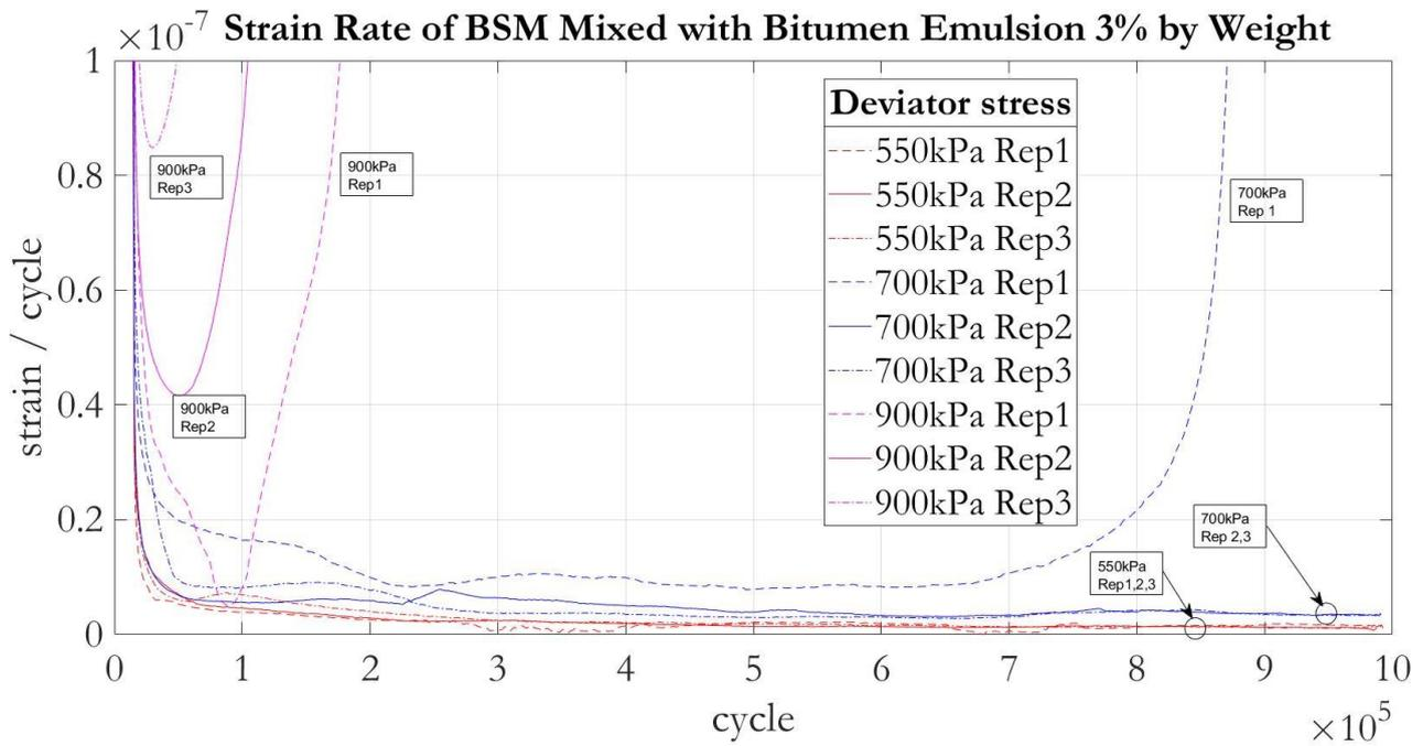
Fig. 8. Relationships between the number of repeated load cycles and the permanent strain rate of the 3% BSM specimens.
