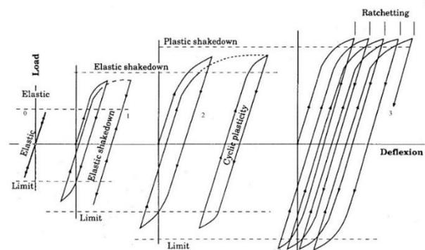
Fig. 1. Patterns of material behavior under repeated loads [19].
