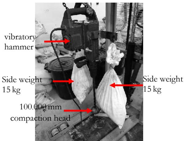
Fig. 4. Vibratory hammer used in compaction.
