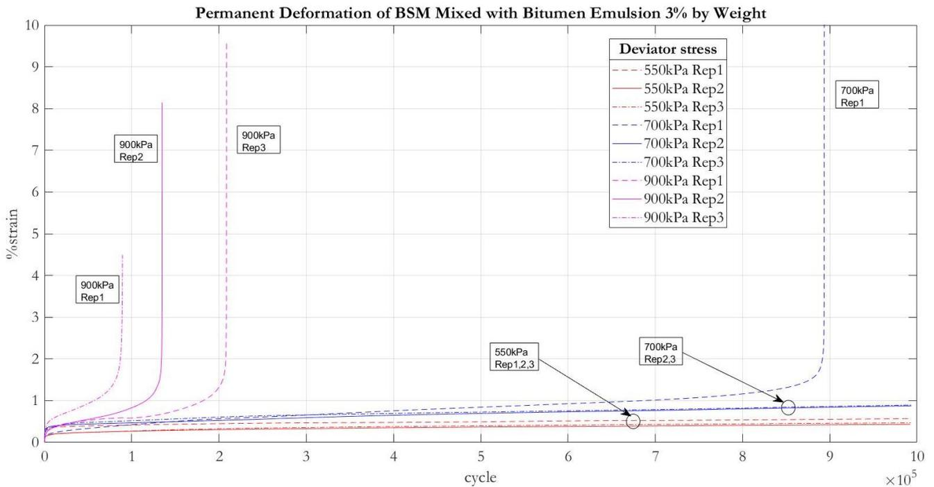
Fig. 7. Relationships between the number of repeated load cycles and the accumulated permanent strain of the 3% BSM specimens.
