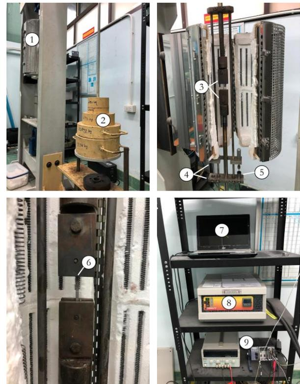
Fig. 2. Creep test machine and accessories equipment; (1) Furnace chamber, (2) Dead-weight plates and loading pan, (3) Pin-type grips, (4) Extensometer, (5) LVDT, (6) Specimen, (7) Computer, (8) Furnace temperature.
