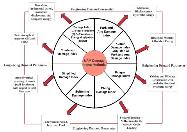
Fig. 3. URM damage index methods and their engineering demand parameters (EDPs).
