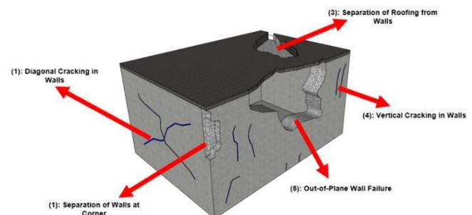
Fig. 1. Types of URM failure mechanism.
