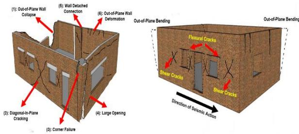
Fig. 2. Common failure mechanism for adobe masonry structures.
