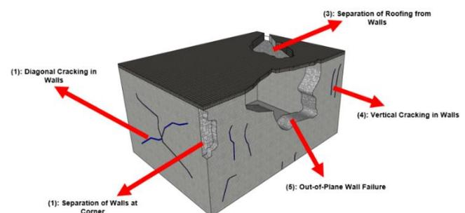
Fig. 1. Types of URM failure mechanism.
