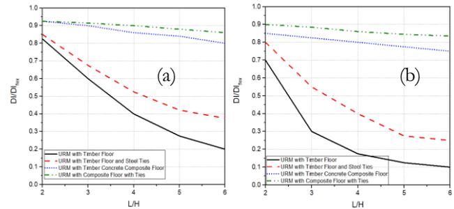
Fig. 5. Diagram relating  $DI/D_{flex}$  to  $(1/h)$  for URM buildings up to three storeys, (a)  $0.15 < f_t < 0.25$  MPa, (b)  $f_t < 0.15$  MPa reproduced from Morić [71].
