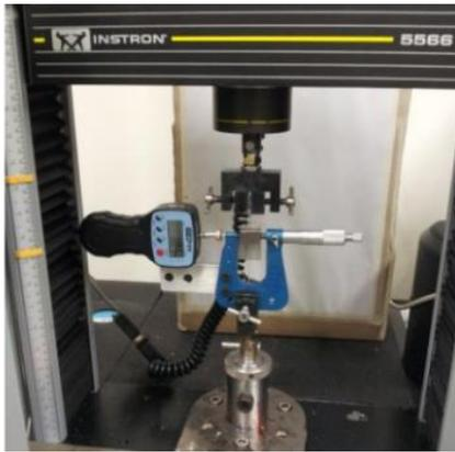
Fig. 2. The strip drawing test to measure the friction coefficient of AA1235.
