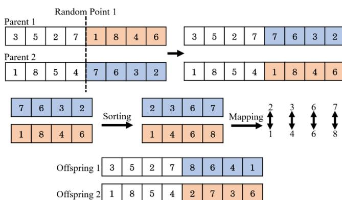
Fig. 5. Example of Weight Mapping Crossover (WMX).
