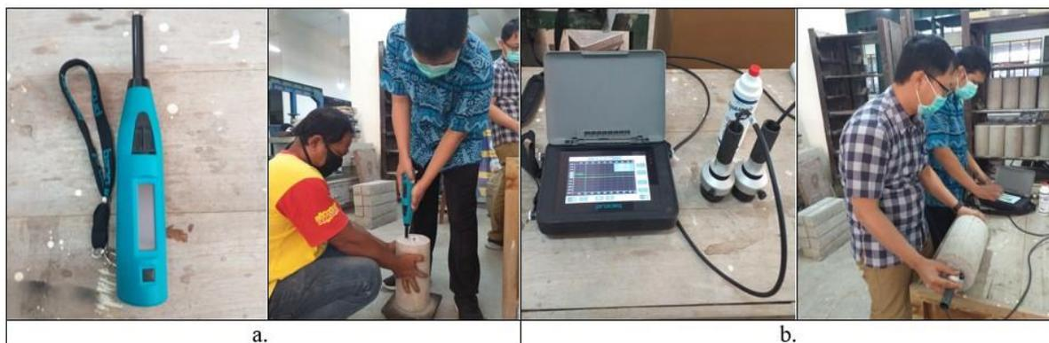
Fig. 3. Non-destructive testings: a. Schmidt's hammer test b. Ultrasonic Pulse Velocity test.
