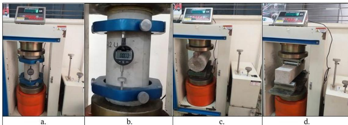
Fig. 2. Destructive testings: a. and b. Compressive test c. Splitting tensile test d. Bending test.
