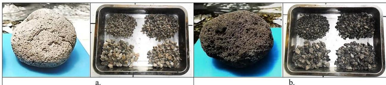
Fig. 1. Four grains sizes of design gradation: a. Pumice and b. Scoria.
