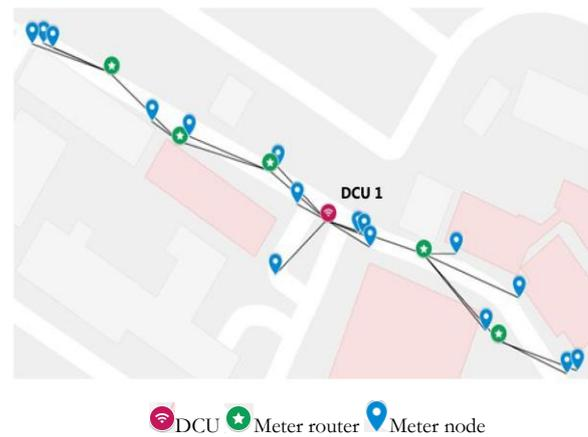
Fig. 5. AMI network topology for DCU location 1.
