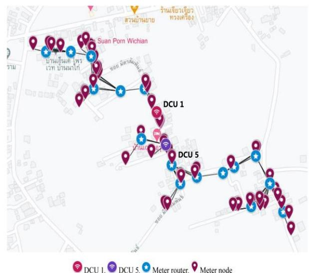
Fig. 12. AMI network topology for 2 DCUs at DCU location 1 and location 5 in the rural area, Nong Khai Province.
