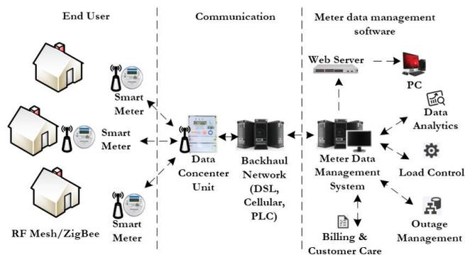
Fig. 1. The architecture of an advanced metering infrastructure (AMI) system.
