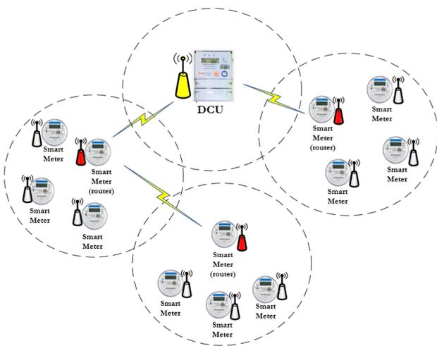
Fig. 2. Advanced metering infrastructure (AMI) network topology.
