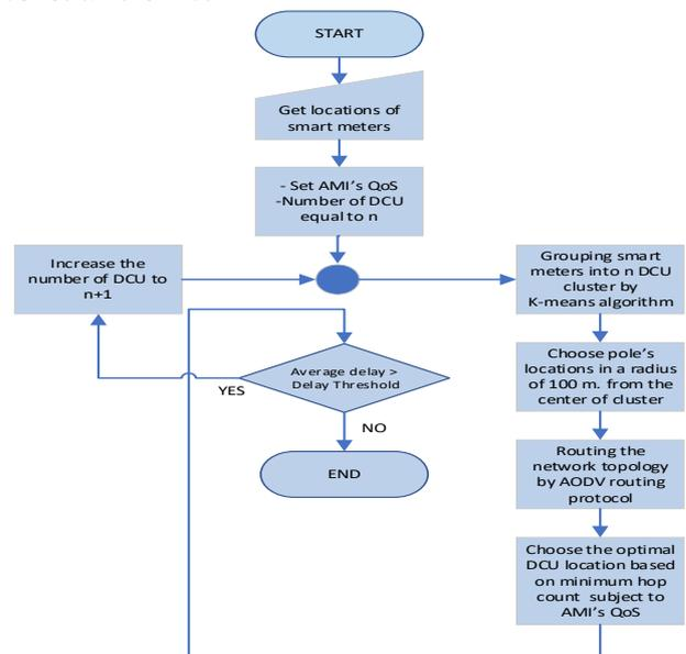
Fig. 3. A flowchart of the proposed optimal DCU placement algorithm.
