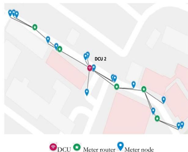
Fig. 6. AMI network topology for DCU location 2.
