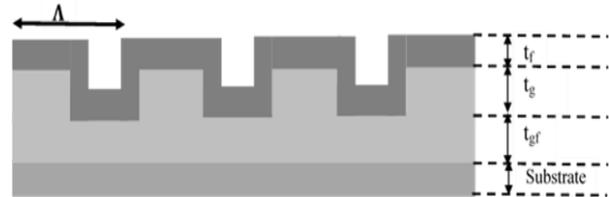
Fig. 2.2 Structure of GMR simulated in RCWA.
