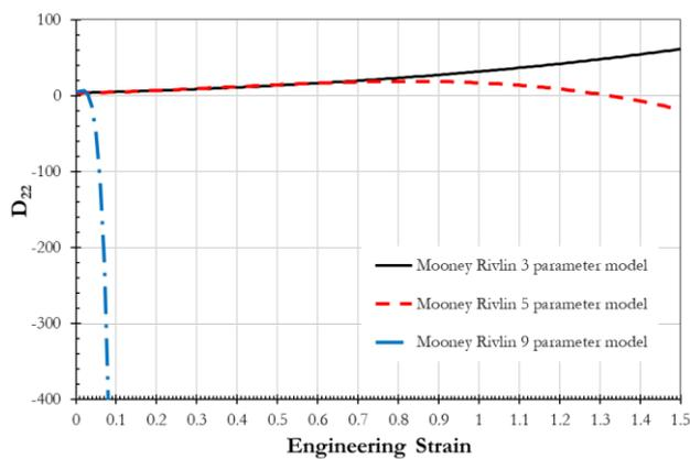
Fig. 29. Plot of  $D_{22}$  and engineering strain for various Mooney-Rivlin models by the *PP* algorithm.
