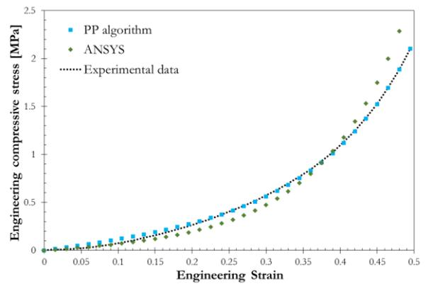
Fig. 18. Comparison of compressive stress-strain curves reproduced from the *PP* algorithm and the ANSYS program by the Yeoh 2<sup>nd</sup> order model to the compressive testing data.
