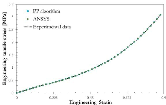
Fig. 12. Comparison of tensile stress-strain curves reproduced from the *PP* algorithm and the ANSYS program by the Mooney-Rivlin 9 parameters model to the tensile testing data.
