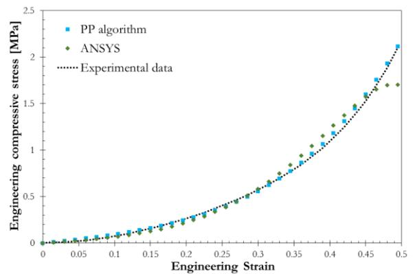
Fig. 19. Comparison of compressive stress-strain curves reproduced from the *PP* algorithm and the ANSYS program by the Yeoh 3<sup>rd</sup> order model to the compressive testing data.
