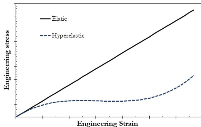
Fig. 1. Engineering stress-strain curves of elastic and hyperelastic materials.
