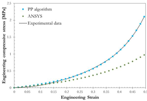
Fig. 25. Comparison of compressive stress-strain curves reproduced from the *PP* algorithm and the ANSYS program by the Ogden 3<sup>rd</sup> order model to the compressive testing data.
