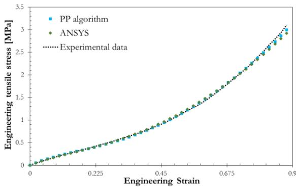
Fig. 10. Comparison of tensile stress-strain curves reproduced from the *PP* algorithm and the ANSYS program by the Mooney-Rivlin 3 parameters model to the tensile testing data.
