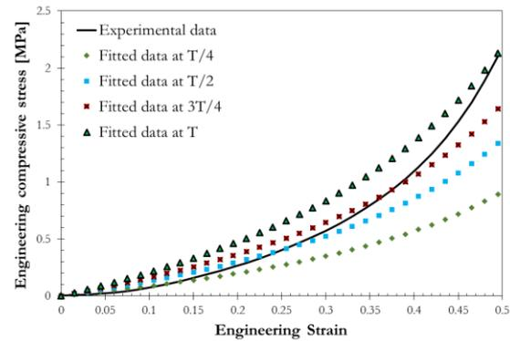
Fig. 7. Comparison of compressive stress-strain curves reproduced from the *PP* algorithm by the Neo-Hookean model to the compressive testing data.
