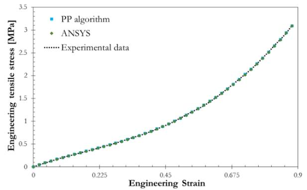
Fig. 22. Comparison of tensile stress-strain curves reproduced from the *PP* algorithm and the ANSYS program by the Ogden 3<sup>rd</sup> order model to the tensile testing data.
