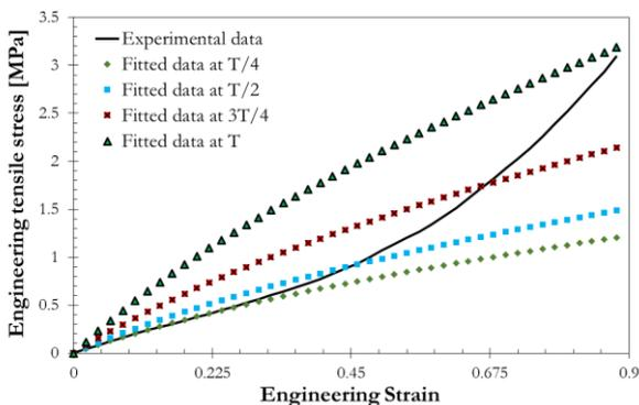
Fig. 6. Comparison of tensile stress-strain curves reproduced from the *PP* algorithm by the Neo-Hookean model to the tensile testing data.
