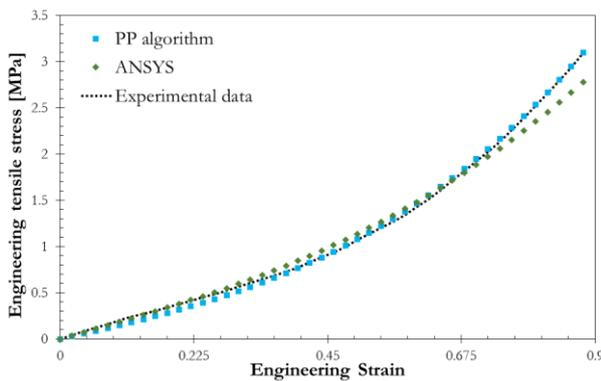
Fig. 20. Comparison of tensile stress-strain curves reproduced from the *PP* algorithm and the ANSYS program by the Ogden 1<sup>st</sup> order model to the tensile testing data.
