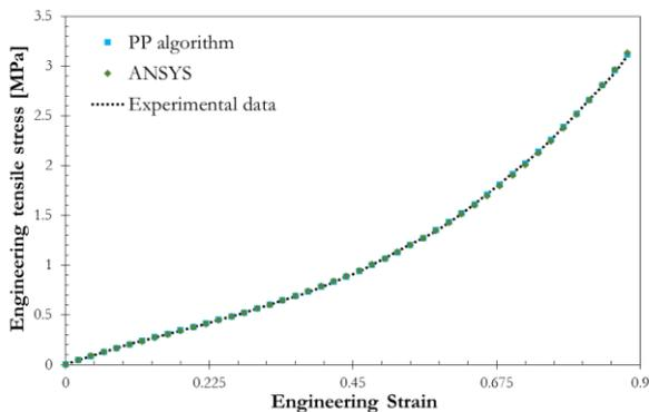
Fig. 11. Comparison of tensile stress-strain curves reproduced from the *PP* algorithm and the ANSYS program by the Mooney-Rivlin 5 parameters model to the tensile testing data.
