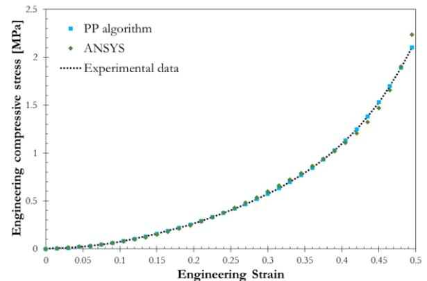
Fig. 14. Comparison of compressive stress-strain curves reproduced from the *PP* algorithm and the ANSYS program by the Mooney-Rivlin 5 parameters model to the compressive testing data.
