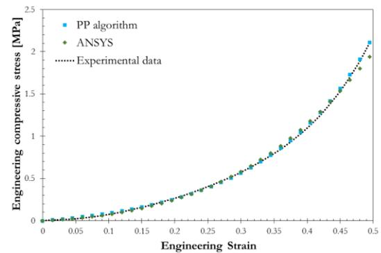
Fig. 13. Comparison of compressive stress-strain curves reproduced from the *PP* algorithm and the ANSYS program by the Mooney-Rivlin 3 parameters model to the compressive testing data.
