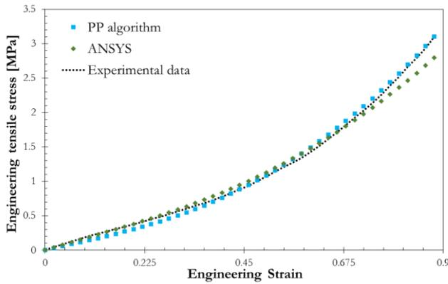
Fig. 16. Comparison of tensile stress-strain curves reproduced from the *PP* algorithm and the ANSYS program by the Yeoh 2<sup>nd</sup> order model to the tensile testing data.
