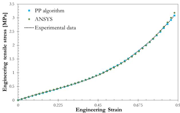
Fig. 17. Comparison of tensile stress-strain curves reproduced from the *PP* algorithm and the ANSYS program by the Yeoh 3<sup>rd</sup> order model to the tensile testing data.
