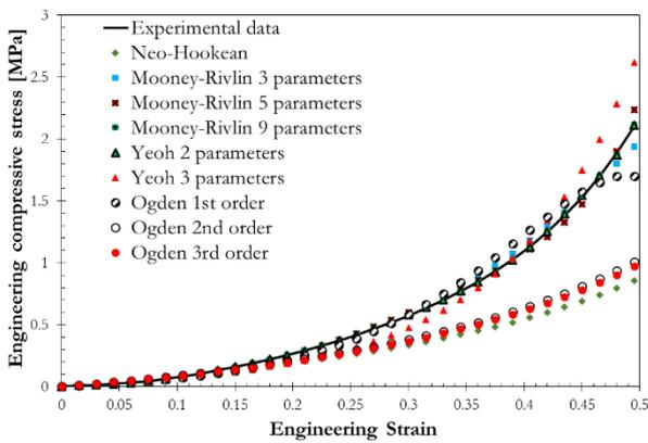
Fig. 4. Comparison of engineering compressive stress and strain curve obtained from the experimental data and various constitutive models by the ANSYS program.
