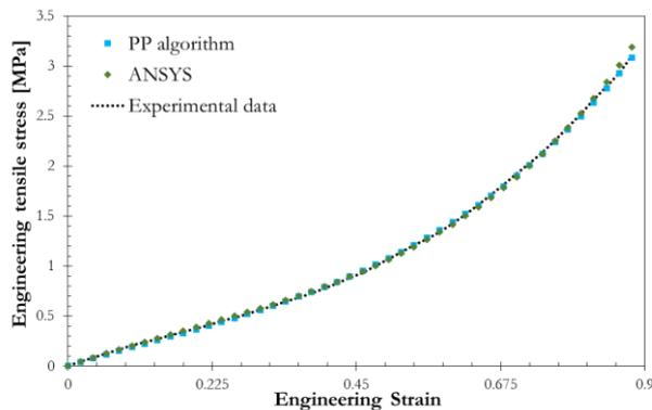
Fig. 21. Comparison of tensile stress-strain curves reproduced from the *PP* algorithm and ANSYS program by the Ogden 2<sup>nd</sup> order model with the tensile testing data.
