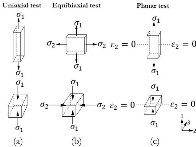
Fig. 2. Hyperelastic material testing: (a) uniaxial test, (b) equibiaxial test, and (c) planar test.
