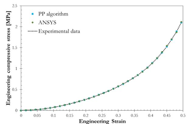
Fig. 15. Comparison of compressive stress-strain curves reproduced from the *PP* algorithm and the ANSYS program by the Mooney-Rivlin 9 parameters model to the compressive testing data.
