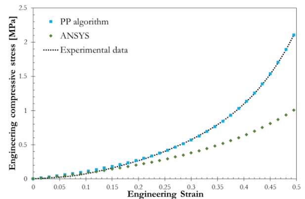
Fig. 23. Comparison of compressive stress-strain curves reproduced from the *PP* algorithm and the ANSYS program by the Ogden 1<sup>st</sup> order model to the compressive testing data.
