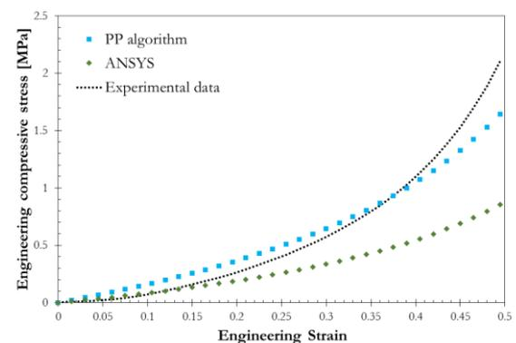
Fig. 9. Comparison compressive stress-strain curves reproduced from the *PP* algorithm (with fitted data at  $3T/4$ ) and the ANSYS program by the Neo-Hookean model to the compressive testing data.
