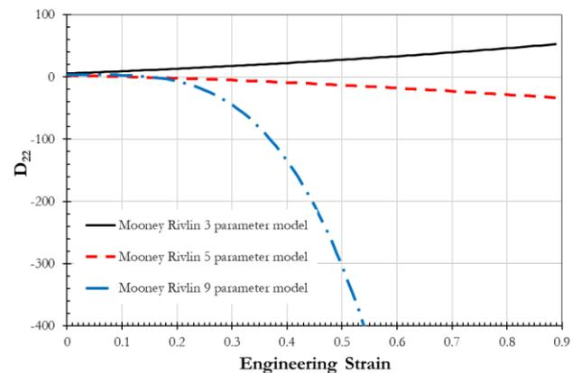
Fig. 28. Plot of  $D_{22}$  and engineering strain for various Mooney-Rivlin models by the *PP* algorithm.
