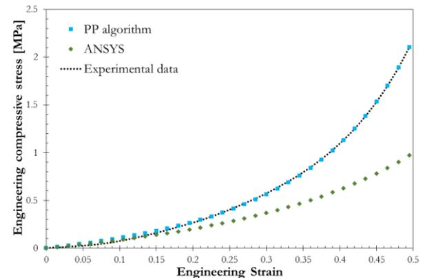
Fig. 24. Comparison of compressive stress-strain curves reproduced from the *PP* algorithm and the ANSYS program by the Ogden 2<sup>nd</sup> order model to the compressive testing data.
