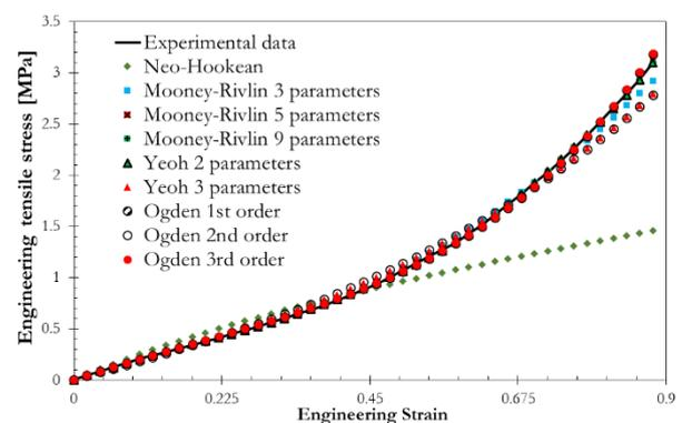
Fig. 3. Comparison of engineering tensile stress and strain
