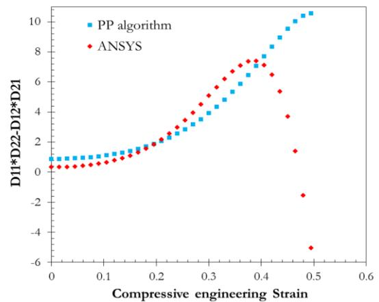
Fig. 27. Comparison  $D_{11}D_{22} - D_{12}D_{21}$  of the Yeoh 3<sup>rd</sup> order model obtained from the *PP* algorithm and the ANSYS program.
