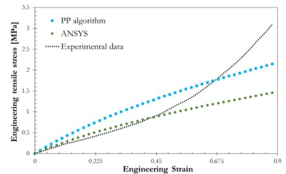
Fig. 8. Comparison of tensile stress-strain curves reproduced from the *PP* algorithm (with fitted data at  $3T/4$ ) and the ANSYS program by the Neo-Hookean model to the tensile testing data.
