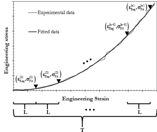
Fig. 5. Selection of the engineering stress-strain data.
