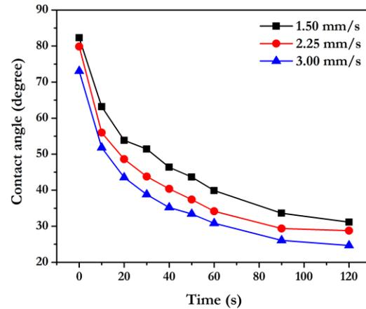
Fig. 9. Contact angle of PEDOT:PSS films prepared with different velocity.
