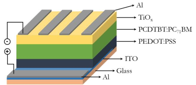
Fig. 3. Schematic structure of OPVs.
