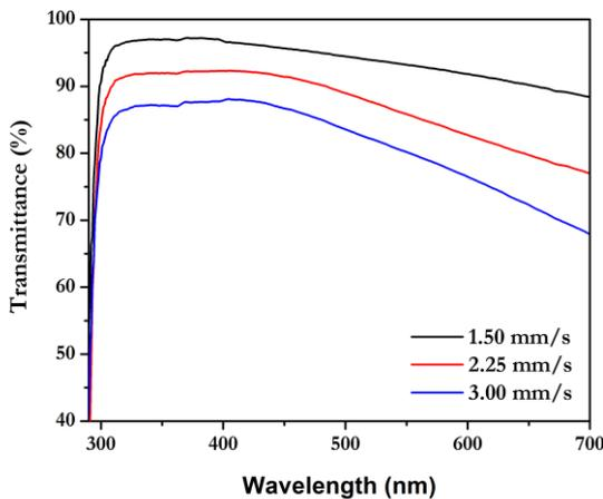
Fig. 7. Transmittance of PEDOT:PSS films prepared at different velocities.
