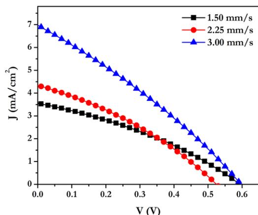
Fig. 10. J-V curves of OPVs fabricated with PEDOT:PSS at different velocities.
