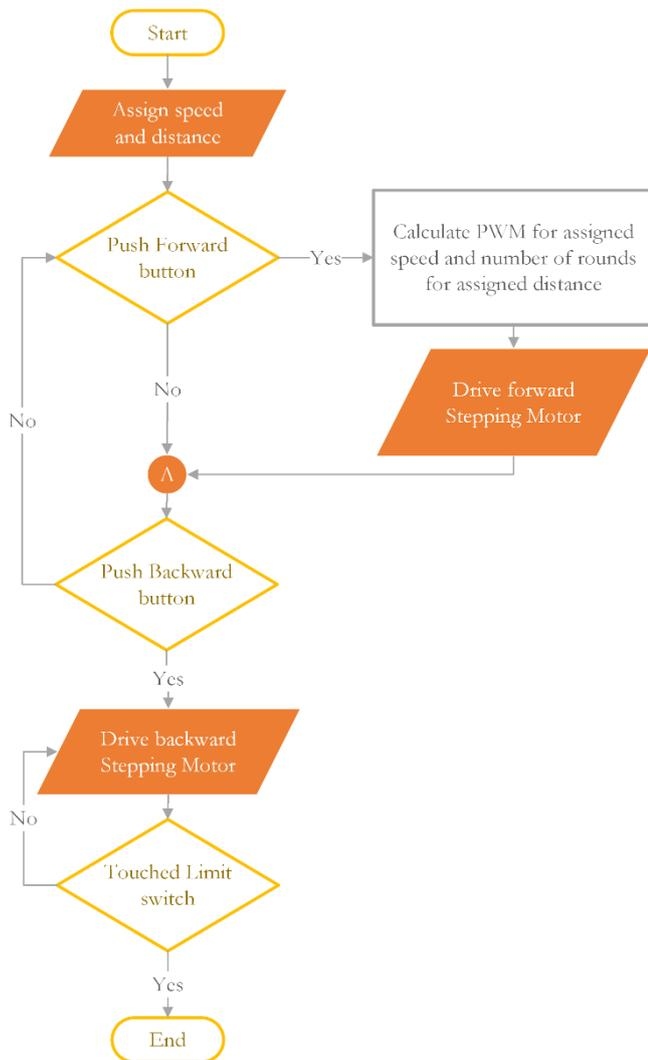
Fig. 2. Flowing chart diagram of Arduino processing.
