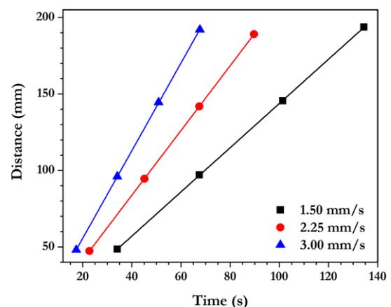
Fig. 4. Distance versus time curves of convective deposition system at different desired velocities.
