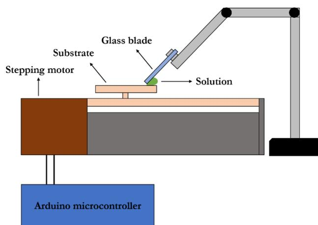
Fig. 1. Schematic structure of convective deposition system.
