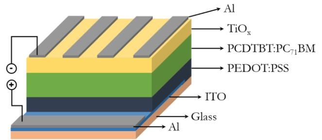
Fig. 3. Schematic structure of OPVs.
