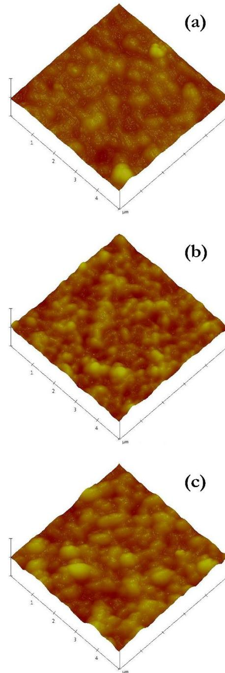
Fig. 5. Topological image of PEDOT:PSS films prepared at convection velocity of (a) 1.50 mm/s, (b) 2.25 mm/s, and (c) 3.00 mm/s.
