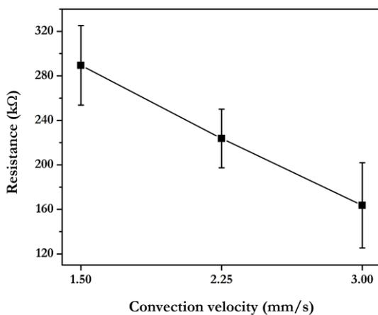
Fig. 8. Resistance of PEDOT:PSS films prepared at different velocities.
