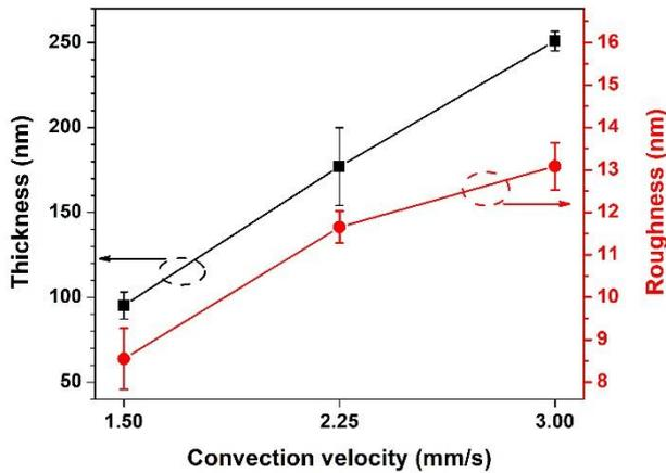
Fig. 6. Relation of thickness and roughness of PEDOT:PSS films prepared at different convection velocities.
