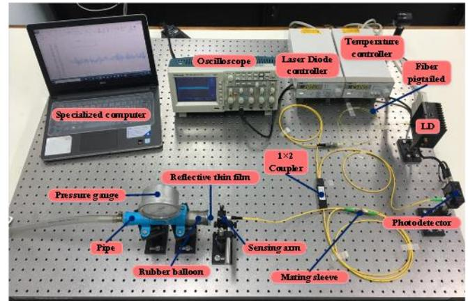
Fig. 8. Experimental setup of EFFPI system for low-pressure measurement application.
