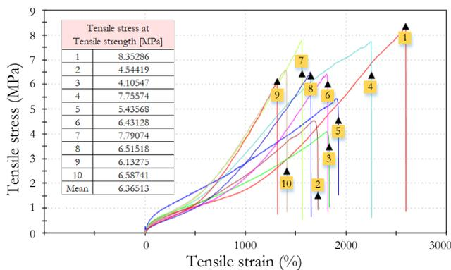
Fig. 7. Testing results obtained from tensile machine.
