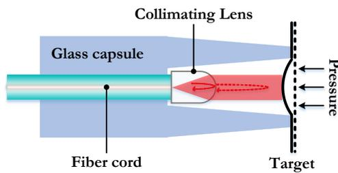
Fig. 3. Example of an optical fiber sensor applied for pressure measurement [27].
