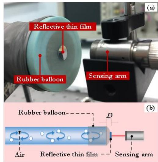
Fig. 9. Schematic of; (a) sensing arm and rubber balloon positioning; (b) airflow directions in target system.
