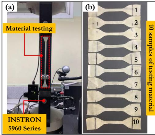
Fig. 6. Examples of material elasticity testing of rubber balloon; (a) material testing by using tensile machine; (b) 10 samples of tested rubber balloon.
