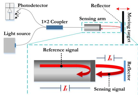
Fig. 1. Basic configuration of EFFPI sensor.
