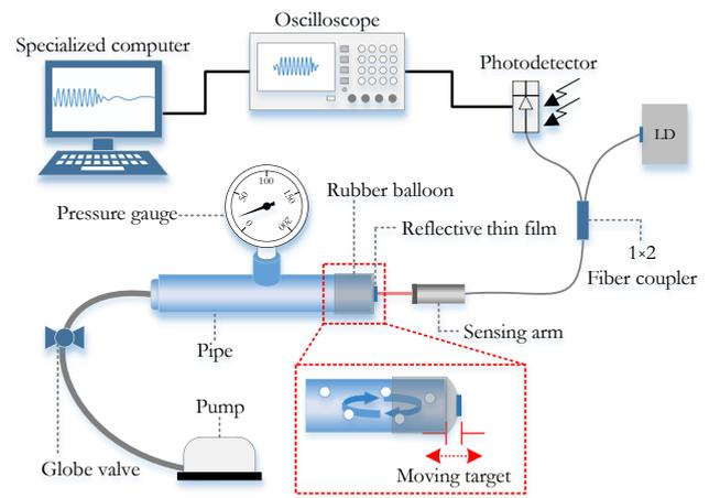
Fig. 5. Configuration of EFFPI measuring system for low-pressure measurement.
