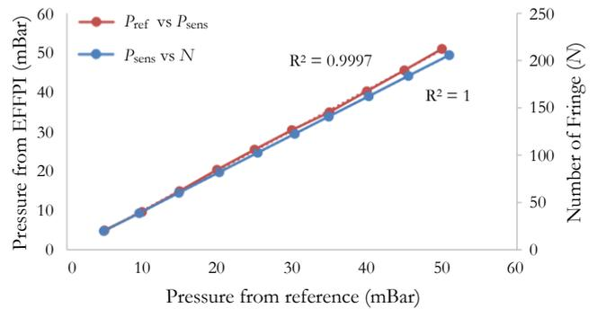
Fig. 11. Comparison of pressure between EFFPI and reference sensor versus number of fringes.
