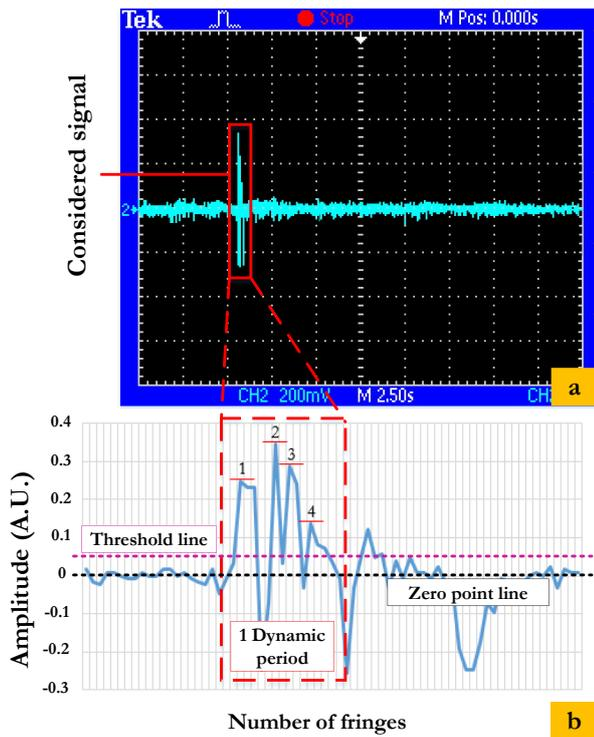
Fig. 10. Output signal obtained from EFFPI sensor; (a) interference signal displayed on oscilloscope and (b) number of fringes via engineering application software.
