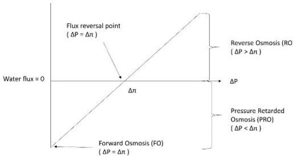
Fig. 2. Directory for the water flux exerted pressure in different condition for FO, PRO and RO.
