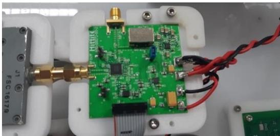
Fig. 6. X-Band Frequency Synthesizer.
