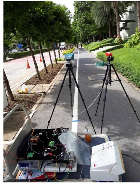
Fig. 16. Field test of X-Band front-end prototype.
