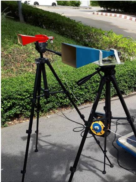
Fig. 15. Transmitted Antenna of PE9856/SF-20 Pasternack model (Blue) and Received Antenna of 3160-07 ETS-Lindgren (Red).
