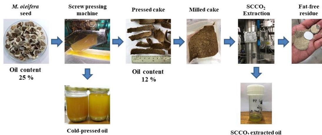
Fig. 2. Schematic of the overall experiment.
