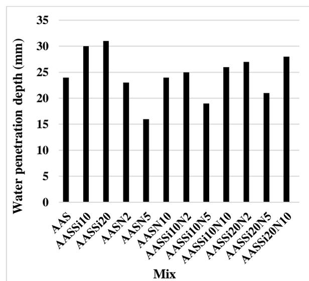
Fig. 8. Depth of water penetration in concrete.
