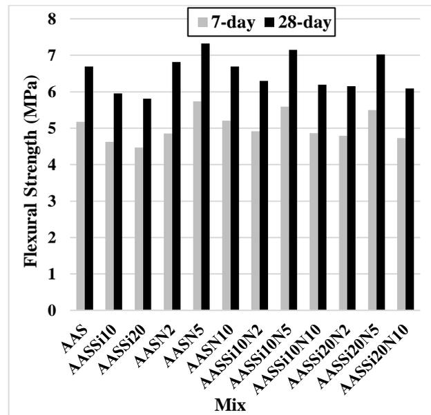
Fig. 2. Comparison of flexural strength of specimens.
