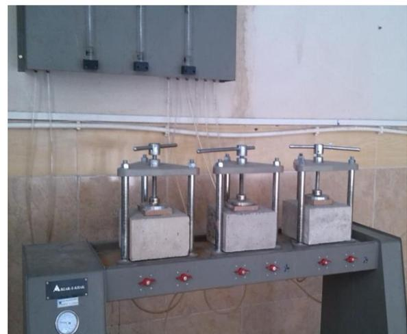
Fig. 7. Depth of water penetration test in concrete.
