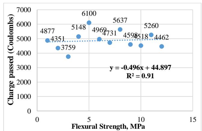
Fig. 11. Relationship between flexural strength and the charge passed of chloride in concrete.
