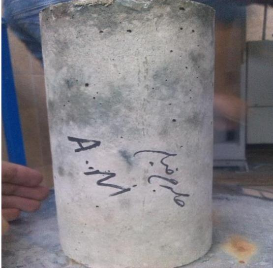
Fig. 3. Compressive specimens.
