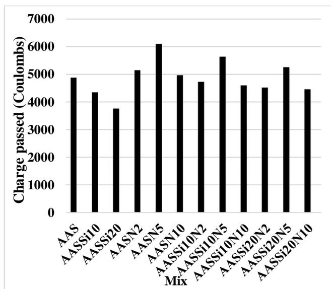
Fig. 6. The charge passed through concrete.
