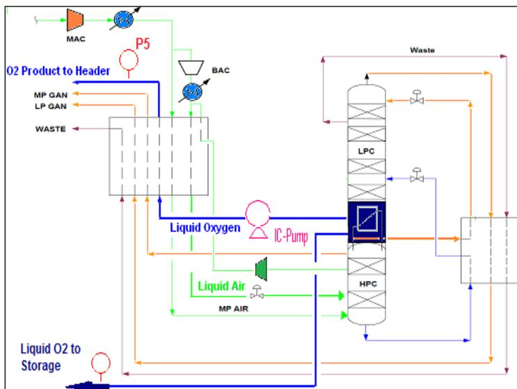
Fig. 7. Locations of O<sub>2</sub> production readings in ASU-71.
