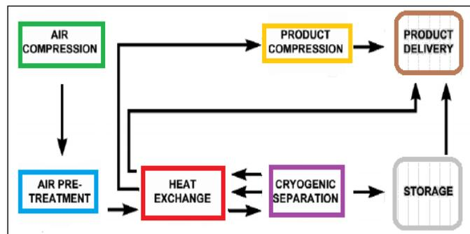
Fig. 2. Units operations for a cryogenic air separation process [13].
