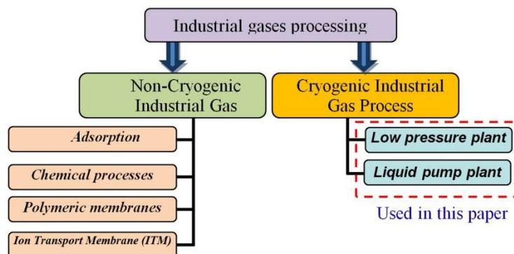
Fig. 3. Classification of industrial gases processing [14].
