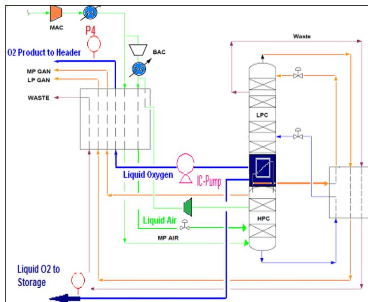
Fig. 6. Location of O<sub>2</sub> production readings in ASU-51.
