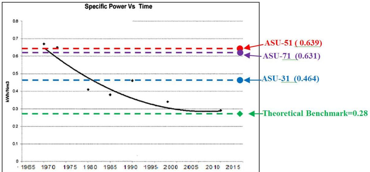
Fig. 8. Benchmarking for O<sub>2</sub> specific power of Air Separation Units.
