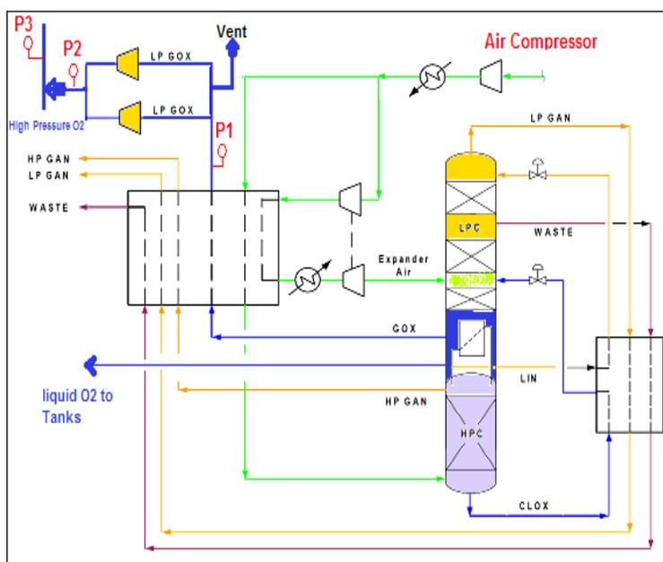
Fig. 5. Locations of O<sub>2</sub> production readings in ASU-31.
