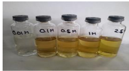
Fig. 3. PLS after heap leaching process using sulfuric acid.
