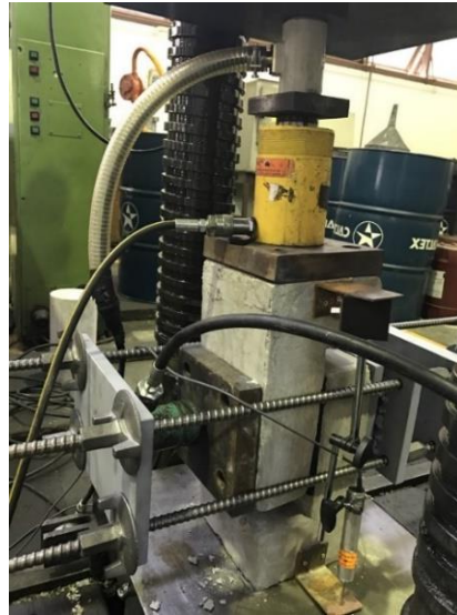
Fig. 4. Compression-shear test; (a) Specimen dimensions in mm; (b) Actual test setup.
