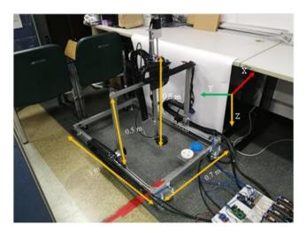
Fig. 3. Structural dimensions of a farming robot.
