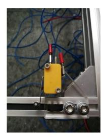
Fig. 8. Installation of limiting switch.
