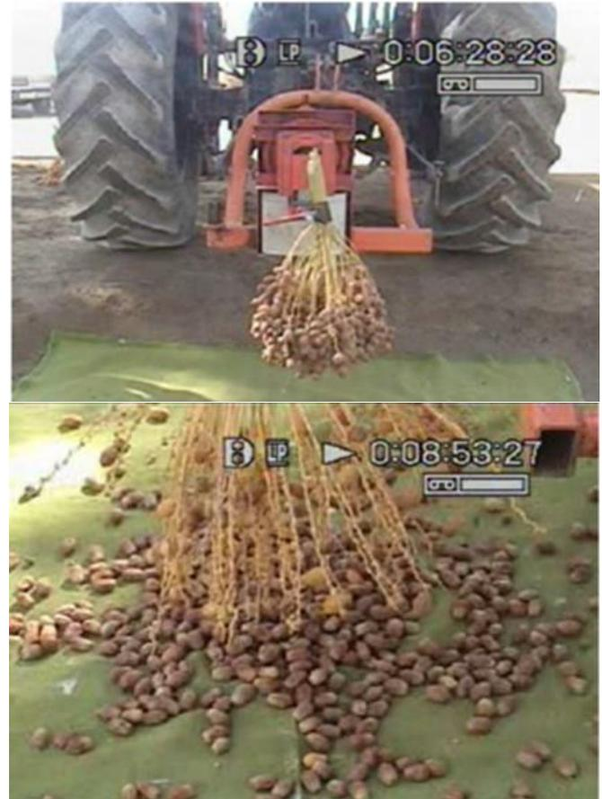
Fig. 1. Tractor-mounted bunch shaker [29].
