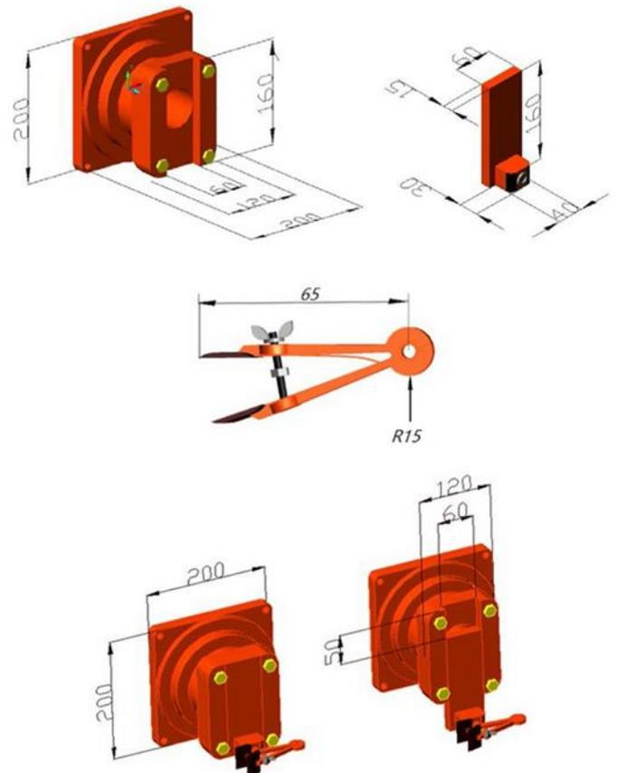
Fig. 7. CAD Modeling of bunch shaker.
