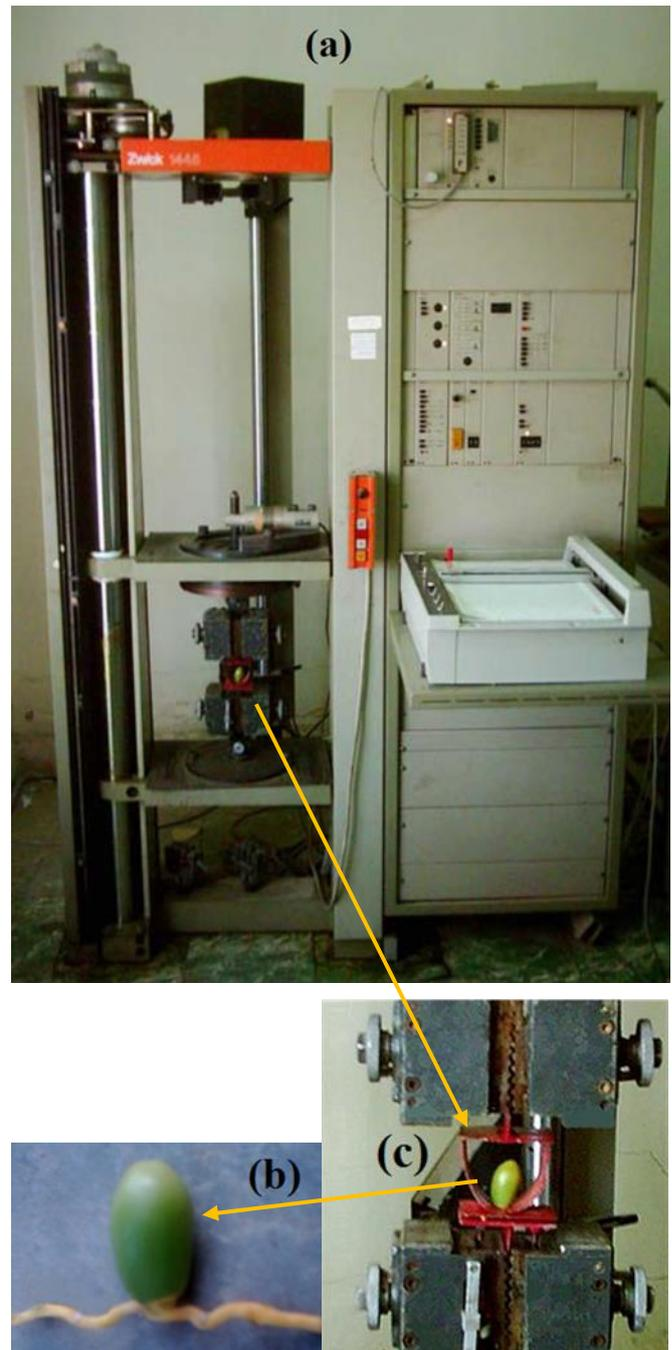
Fig. 9. Static tensile detachment force setup: (a) Universal Testing Machine; (b) test specimen; (c) adapters.
