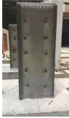
Fig. 3. Reinforcement of the strengthened specimens.
