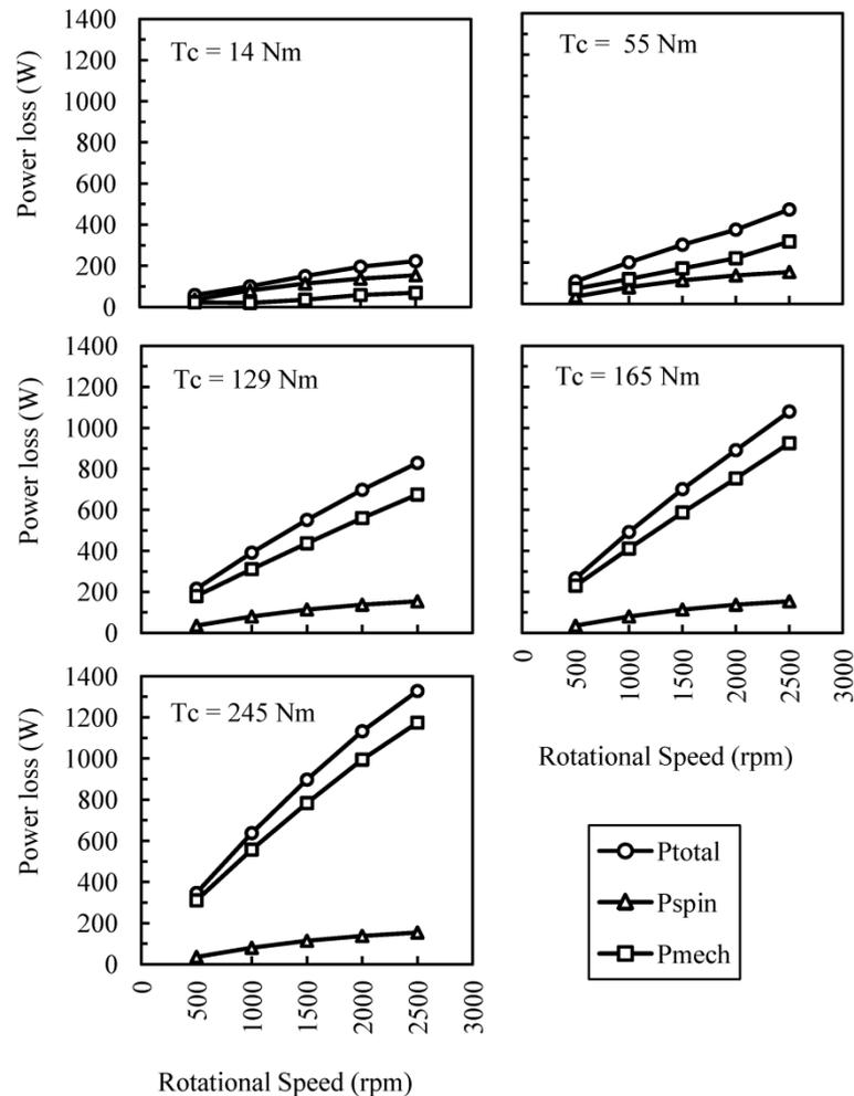
Fig. 6. Measured power losses of gear design 1.
