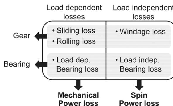
Fig. 4. Category of power losses in the apparatus.
