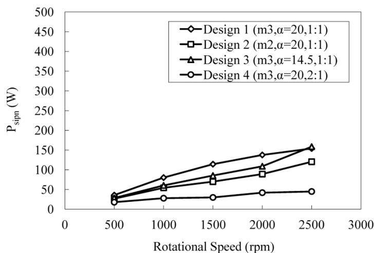
Fig. 5. Measured spin losses.
