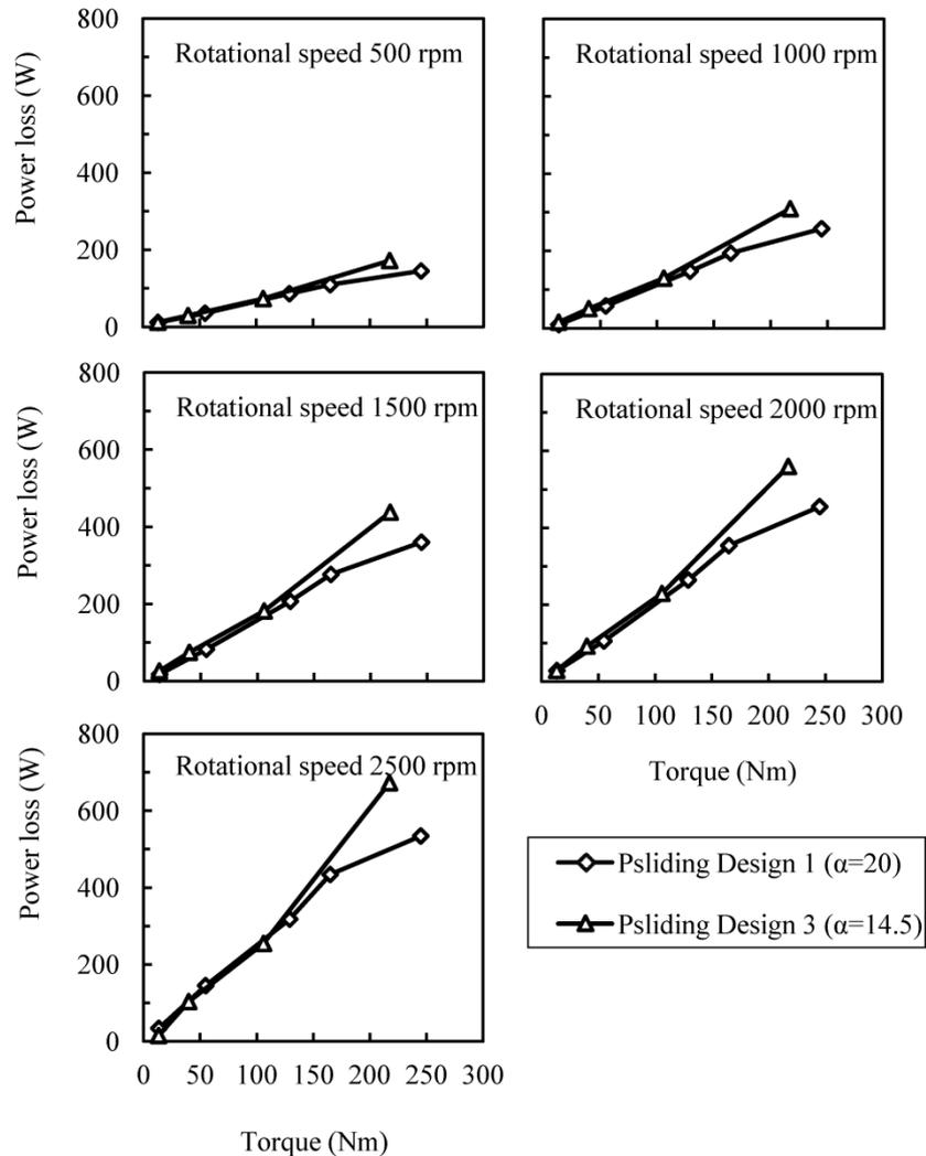
Fig. 9. The effect of pressure angle on the sliding loss.
