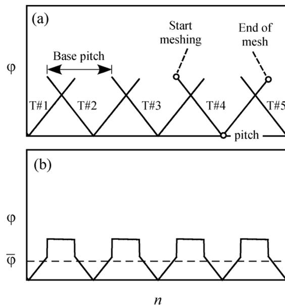
Fig. 1. Sliding loss ratio of a spur gear pair [6].
