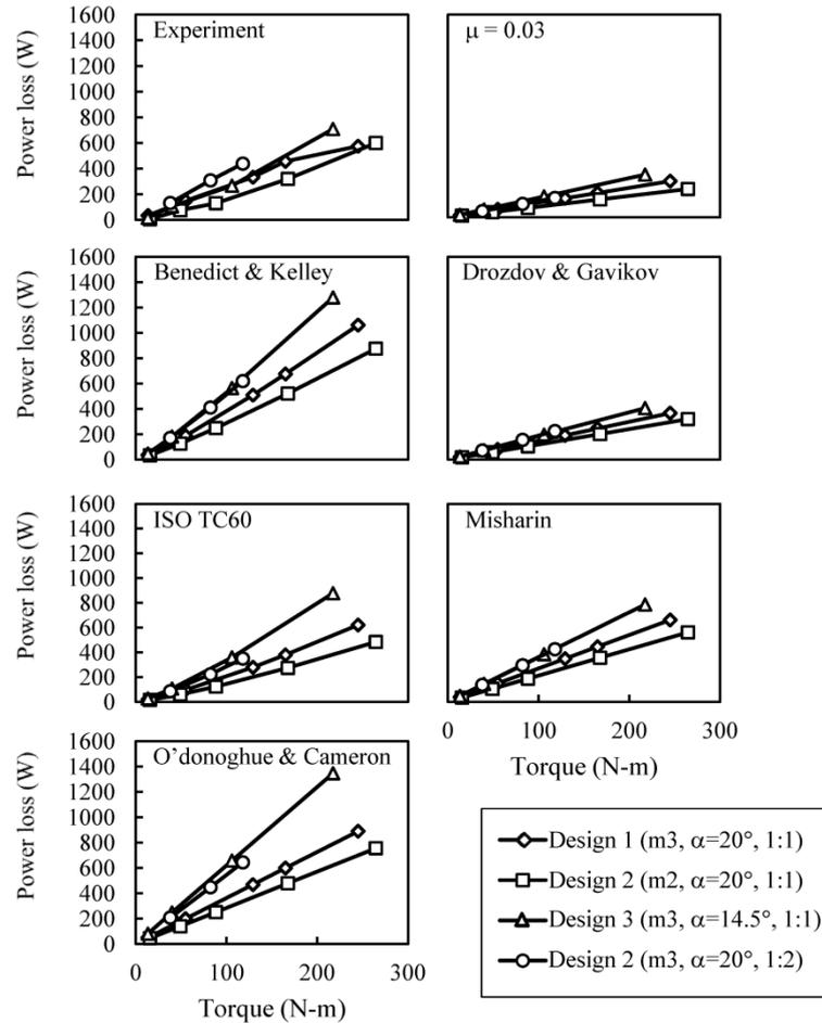
Fig. 11. The estimated sliding loss of various gears at input shaft speed 2500 rpm.
